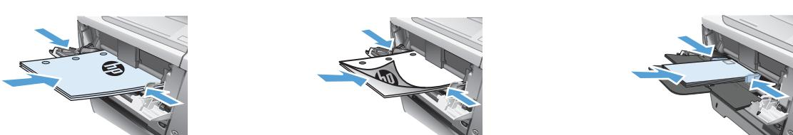
The diagram illustrates three scenarios for loading paper into the 1号纸匣 (Paper Tray 1).
