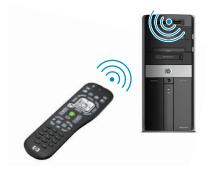
To use the remote control, point it in a direct line of sight at the remote sensor. The remote control and the sensor can be no farther than 8 meters (26 feet) apart. The remote control can be no more than 22.5 degrees (45 degrees total) from the center of the remote sensor.
