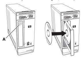
To use a minidisc with a vertical drive, you must first place the computer on its right side (select models only) before you insert the minidisc:
