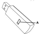
Push the Connect button (**A**) on the receiver (which is also the LED light), and hold it for 5 to 10 seconds until the light starts to flash.
