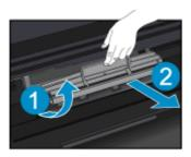
3. Press on the hole of the duplexer path cover to lift it up. Remove the jammed paper.
