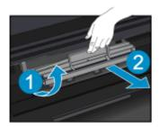
3. Remove the jammed paper from the rear roller.
