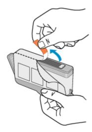
**b**. Twist the orange cap to snap it off. A forceful twist may be required to remove the cap.
