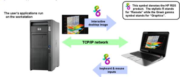
The workstation image is transmitted over the network to the receiver, which displays the desktop image locally in a window. RGS is designed to provide fast capture, compression, and transmission of the desktop image over standard TCP/IP networks. RGS also captures user keyboard and mouse inputs from the client and sends them over the network to the sender.
