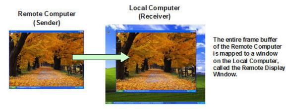
In <u>Figure 2-4 Display of the Remote Computer frame buffer on the Local Computer on page 17</u>, the Remote Computer frame buffer fits completely within the Remote Display Window on the Local Computer monitor. However, it is possible for the Remote Computer frame buffer size to exceed the
