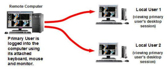
In <u>Figure 2-8 Sharing between workstations on page 20</u>, the primary user is directly logged into the Remote Computer using its attached keyboard, mouse and monitor. In other words, the primary user is physically present at the Remote Computer, while local user 1 and local user 2 are physically separate
