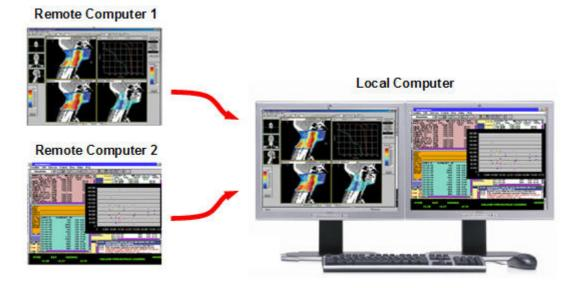
As always, each Remote Computer (Sender) frame buffer is displayed in its own Remote Display Window. In <u>Figure 2-16 Each Remote Display Window can be positioned to occupy a single monitor on page 27</u>, the user has positioned each Remote Display Window to occupy a single monitor, achieving the result that the left monitor is dedicated to Remote Computer 1 while the right monitor is dedicated to Remote Computer 2.
