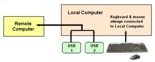
In <u>Figure 2-18 Remote Computer can access the local USB devices on page 30</u>, two USB devices are connected to the Local Computer. Using RGS, the local USB devices can be attached to the Remote Computer. The keyboard and mouse always remain connected to the Local Computer, and cannot be attached to the Remote Computer.
