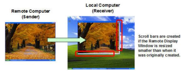
NOTE: RGS does not provide a scale-to-fit capability to allow the contents of the Remote Computer frame buffer to be scaled to fit the Local Computer monitor. If the Remote Computer frame buffer is larger than the Local Computer monitor, the Remote Display Window will simply extend beyond the edges of the monitor. If the Remote Display Window is resized to fit on the monitor, scroll bars will be added.
