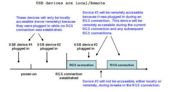
As can be seen in Figure 2-21 USB device accessibility for the setting "USB devices are Local/Remote" on page 33, USB device accessibility depends on when the USB device is plugged into the Local Computer. If a USB device is inserted while no RGS connection is established, the device will be locally-accessible only. If a USB device is inserted while an RGS connection is established, the device will be remotely-accessible only.
