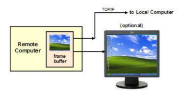
The monitor itself is optional on the Remote Computer. For example, if the Remote Computer is a Personal Workstation, a monitor (plus a keyboard and mouse) would typically be attached. If the Remote Computer is an HP ProLiant Blade Workstation, it is not possible to attach a monitor to view the primary (NVIDIA) frame buffer because the video signal from the NVIDIA graphics adapter is not available on a connector—the contents of the frame buffer can only be viewed remotely using RGS.
