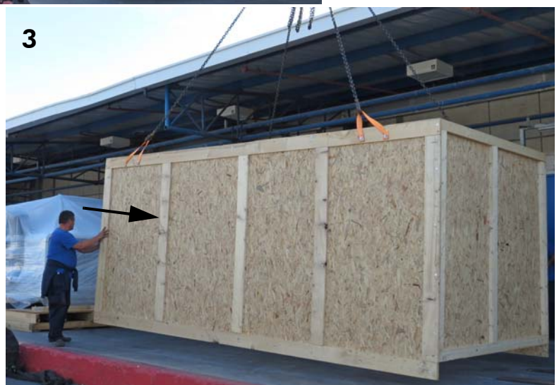
Figure 5-14 Removing Half the Crate Using the Crane
