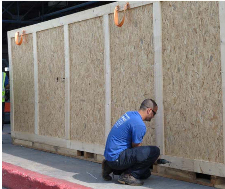
Figure 5-11 Removing Bolts at Bottom of Crate
