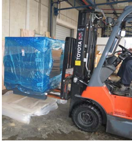
Figure 5-7 Lifting Vacuum Pump from Pallet with Forklift
