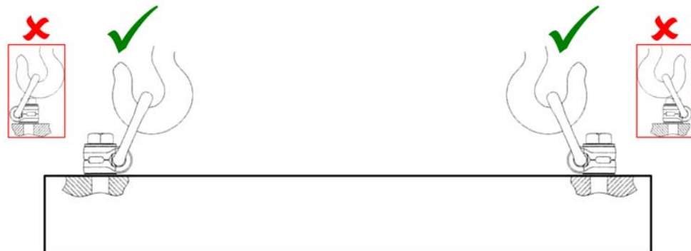
Figure 5-18 Orientation of Eyebolts when Lifting Machine (drawing is not to scale)
