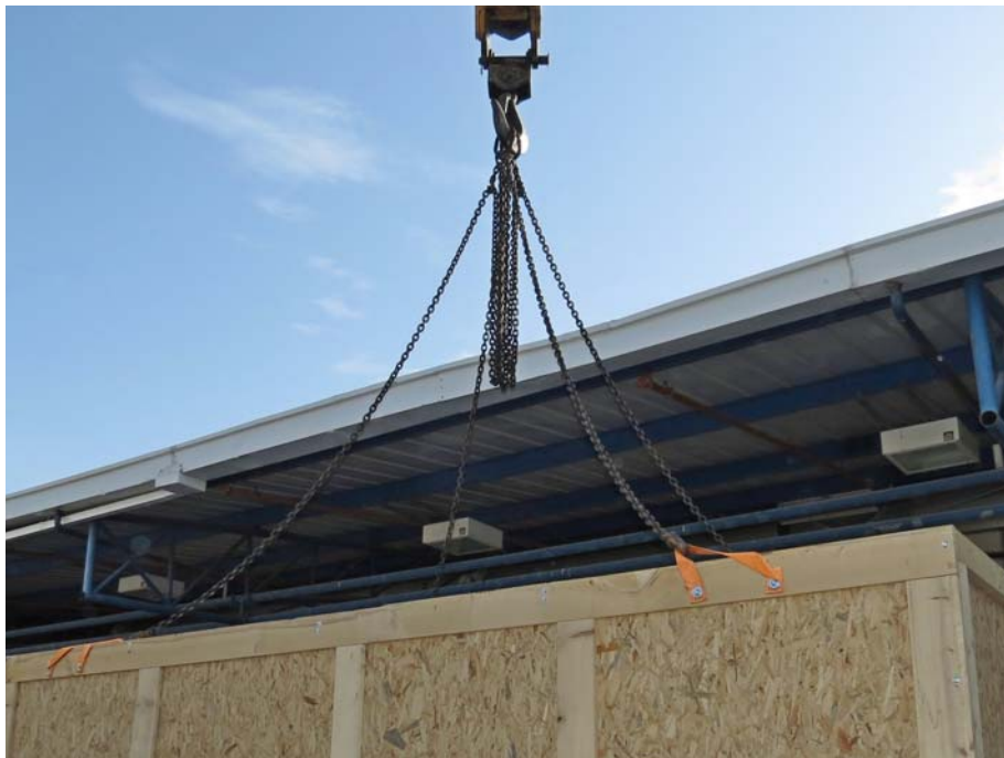
Figure 5-13 Attaching Chains to Crate
