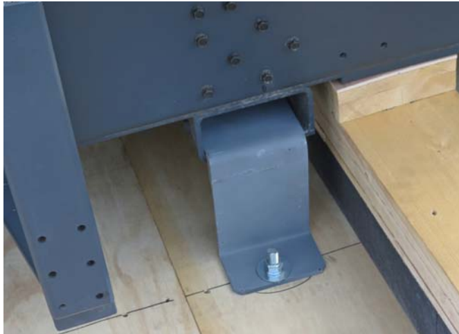
Figure 5-15 Removing Securing Bolts from Pallet
