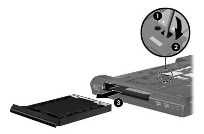
To install an optical drive in the upgrade bay:
