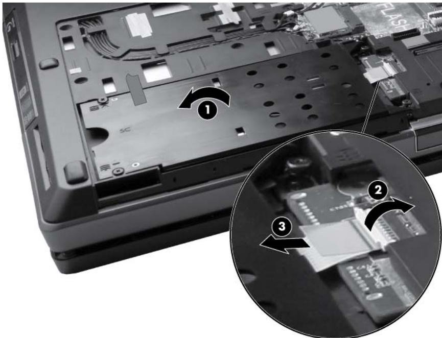
3. Reopen the door (1), and then lift the smart card reader door straight up from the computer (2).
