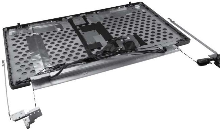
13. If it is necessary to remove the cable routing tray, remove the five Phillips M2.0×3.0 screws **(1)** that secure the cable routing tray to the display enclosure. The cable routing tray is available in the Raw Panel Support Kit, spare part number 657408-001.
