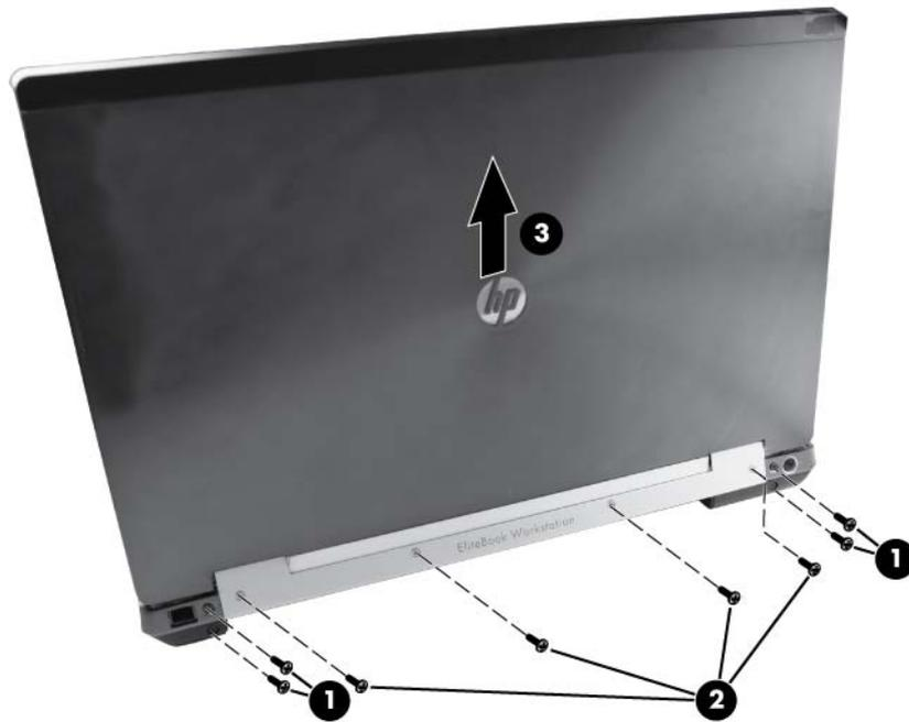
12. If it is necessary to replace the display hinges, remove them from the hinge cover. The left and right display hinges are available using spare part number 652646-001.
