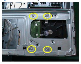
To install a hard drive, reverse the removal procedures.
