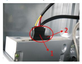
5. Un-screw and slide the drive out the front of the unit. Removing the Optical Drive
