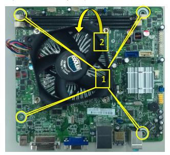
Slide the system board toward the front of the chassis, and then lift the board out of the computer(2).
