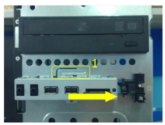
To install the front I/O assembly, reverse the removal procedure.
