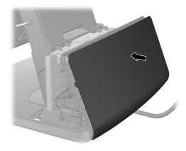
11. Replace the power supply cover by lowering it down over the neck of the base then sliding it back until it snaps in place.
