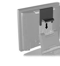
6. Rotate open the small door at the base of the power supply housing **1** and slide the power supply brick into the housing **Q**.
