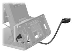
9. Route the cables to peripheral devices underneath the rear of the base, then through the hole in the center of the base, then up through the cable retainer on the neck of the stand and into the appropriate I/O port.
