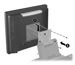
Slide the mounting bracket cover down over the 5. stand's mounting bracket.
