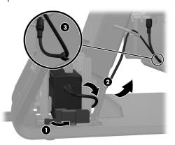
Route the AC power cord through the bottom of 8. the stand's base, then through the cavity inside the base and connect the cord to the power supply brick. Insert the cord into the cable retainer clip on the side of the base and connect the other end of the cord to an electrical outlet.
