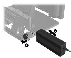
7. Close the small door at the base of the power supply housing **1**. Route the power supply cord through side of the base, then out through the center of the base @ and up through the cable retainer on the neck of the stand. Insert the cord into the cable retainer clip next to the power port 3 and connect the cord to the DC In power port.
