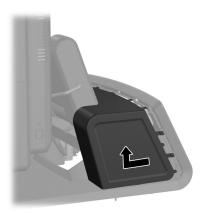
3. Remove the decorative panel on the rear of the unit by gently prying the panel away from the base at the tab locations on the top and sides of the panel as indicated below 1. Then pull the top of the panel away from the base 2 and push straight down on the panel to release the bottom tabs 1.
