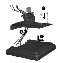
**6.** Slide the cable ends through the hole in the center of the decorative panel that was included with the customer display.
