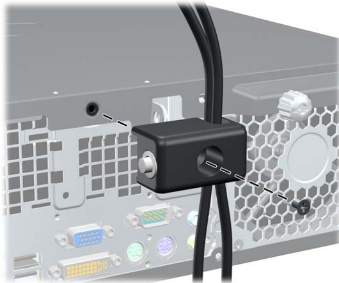
Figure B-9 Attaching the Lock to the Chassis
