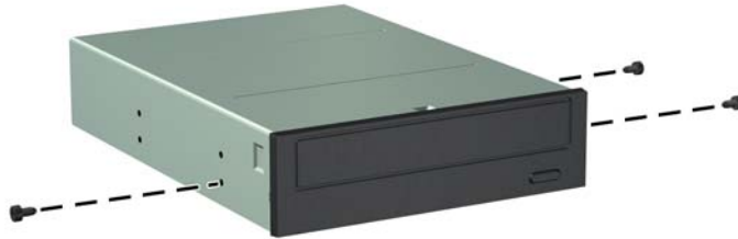
Figure 2-23 Installing Mounting Screws in the Optical Drive
