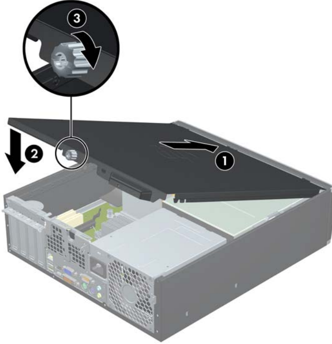
Figure 2-2 Replacing the Access Panel
