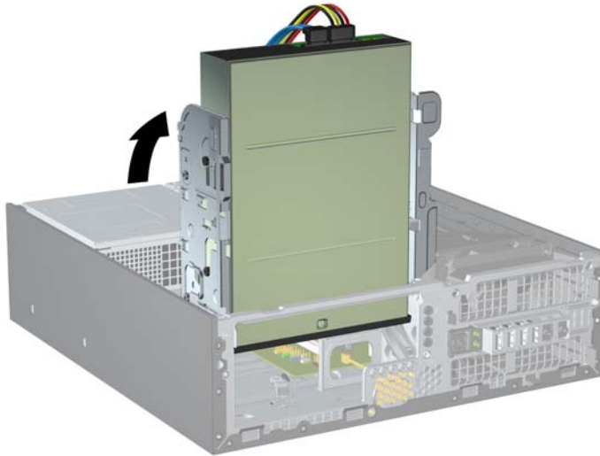
Figure 2-8 Rotating the Drive Cage Up
