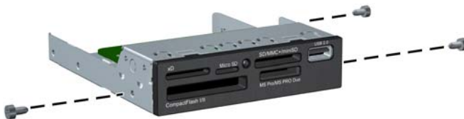
Figure 2-32 Installing Mounting Screws in the Media Card Reader
