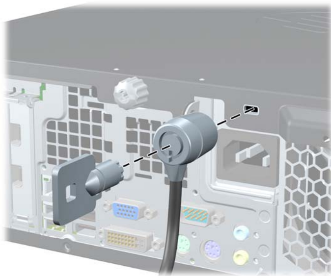
Figure B-1 Installing a Cable Lock
