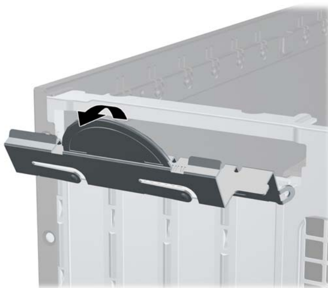
Figure 2-11 Opening the Expansion Slot Retainer
