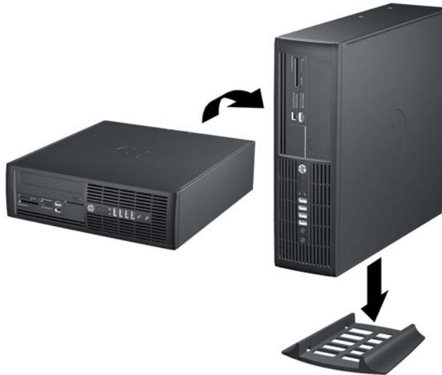
Figure 2-6 Changing from Desktop to Tower Orientation
