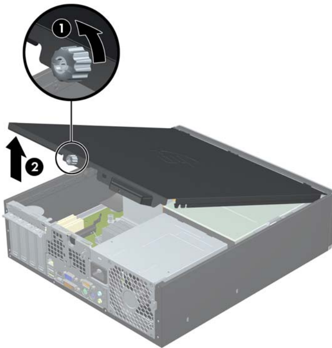
Figure 2-1 Removing the Access Panel
