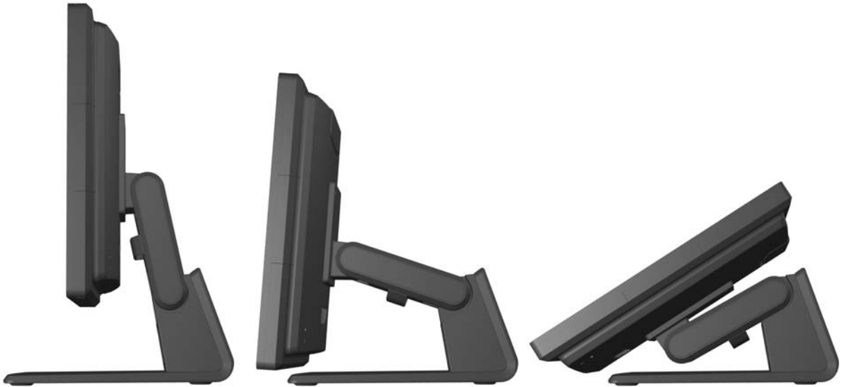
Figure 2-19 Adjusting the Optional Monitor Stand
