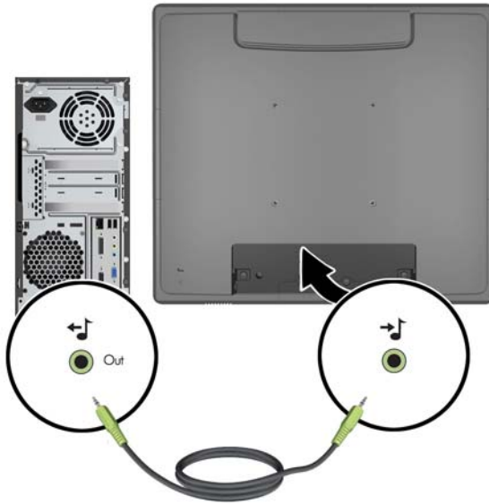
Figure 2-24 Connecting the Audio Cable
