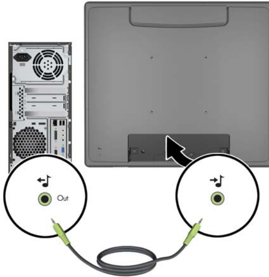
Figure 2-24 Branchement du câble audio
