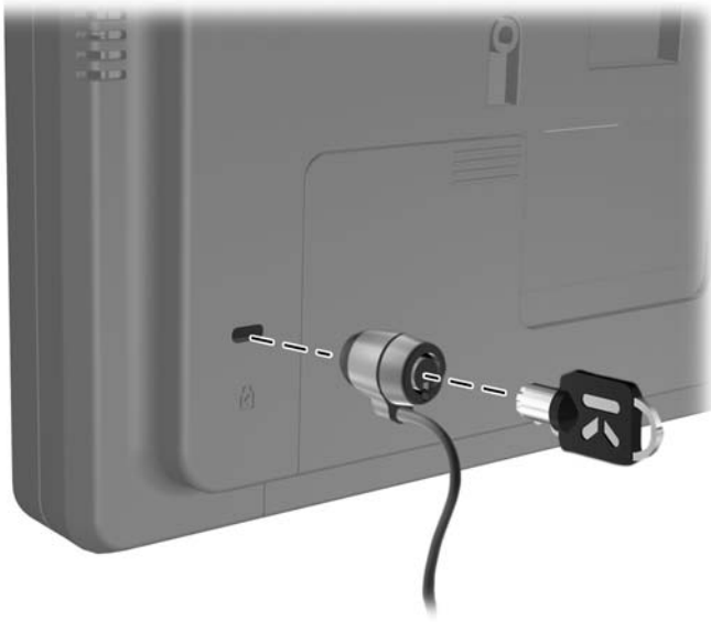
Figure 2-30 Installing a Cable Lock
