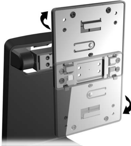
Figure 2-12 Rotating the Mounting Bracket 180°
