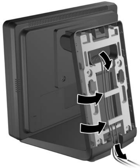
Figure 2-9 Routing the Cables
