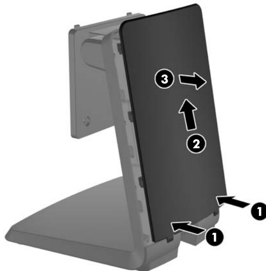
Figure 2-3 Removing the Rear Cover
