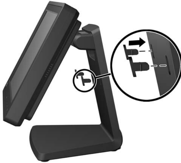
Figure 2-8 Replacing the Access Plugs
