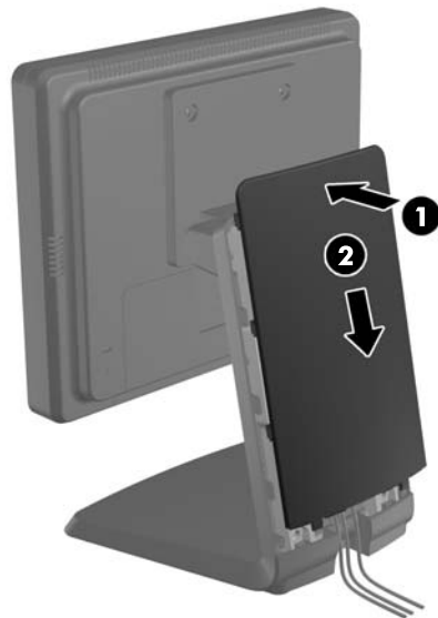
Figure 2-19 Replacing the Rear Cover
