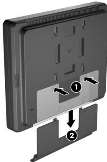
Figure 2-21 Removing the Cable Connection Cover Plate
