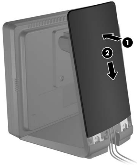
Figure 2-10 Replacing the Rear Cover
