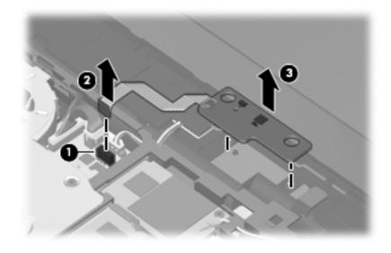
Reverse this procedure to install the power connector board.
