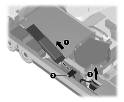
Reverse this procedure to install the Bluetooth module.
