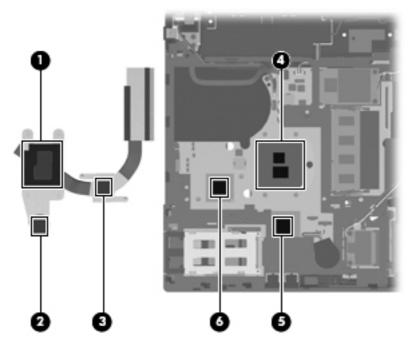
Reverse this procedure to install the heat sink and fan.
