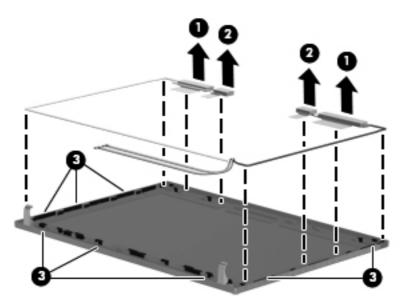
b. Remove the wireless antennas and cables.
