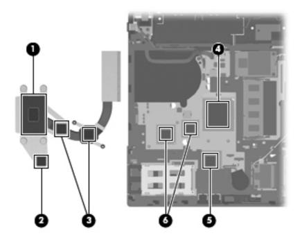
**NOTE:** The thermal material must be thoroughly cleaned from the surfaces of heat sink for the UMA system board (1), (2), and (3) and the system board components (3), (4) and (5) each time the heat sink is removed. Replacement thermal material is included with all heat sink, system board, and processor spare part kits.
