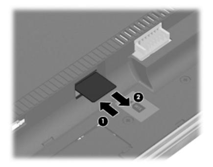
Install the SIM by inserting it into the SIM slot and pushing until you hear a click.
