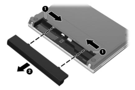
Install the battery by inserting it into the battery bay until you hear a click.
