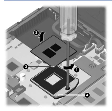
Reverse this procedure to install the processor.
