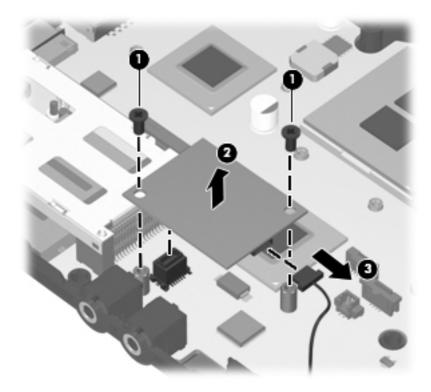
5. Remove the modem module.
