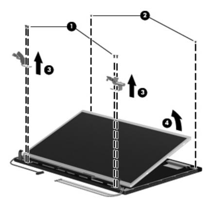
9. Remove the four Phillips PM2.0×3.0 screws (1) that secure the display hinges to the display panel, and then remove the display hinges (2). The left and right display hinges are available in the display hinge kit.
