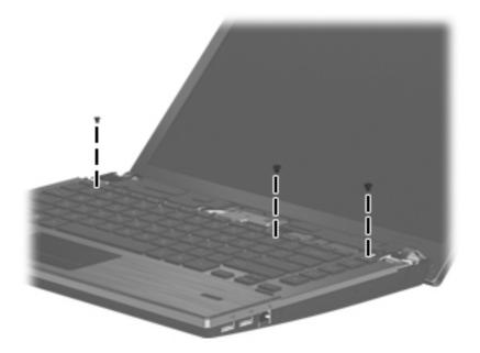
2. Slide the keyboard back toward the display (1), and then rotate it right (2) until it rests upside down on the right side of the computer.
