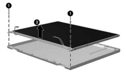
6. Remove the display panel assembly (2) from the display enclosure.
