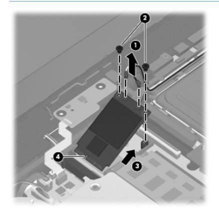
Reverse this procedure to install the WWAN module.
