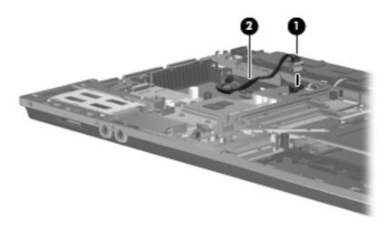
4. Remove the power connector cable
