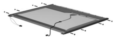
9. Use a sharp-edged tool to cut the tape (1) that secures the sides of the display panel to the display panel frame.
