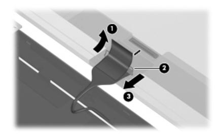
12. Gently pull the integrated microphone (1) from the clips at the top of the display back cover, remove the display cable from the clips and routing channels (2) along the bottom of the display back cover, and then remove the display cable (3). The display/mic/webcam cable is included in the display cable kit.
