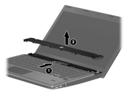
Reverse this procedure to install the switch cover and keyboard.
