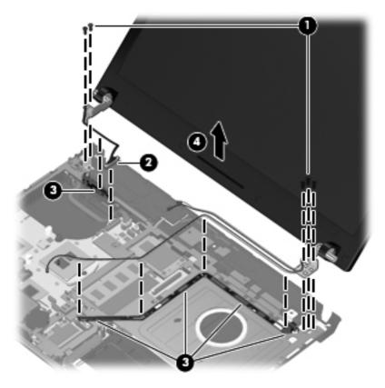
4. If it is necessary to replace the display bezel, display enclosure, or display hinges, remove the four Mylar screw covers (1) and the four T8 slotted-Torx M2.5×6.0 screws (2) that secure the display bezel to the display assembly. The screw covers are available in the rubber kit, spare part number 599564-001.
