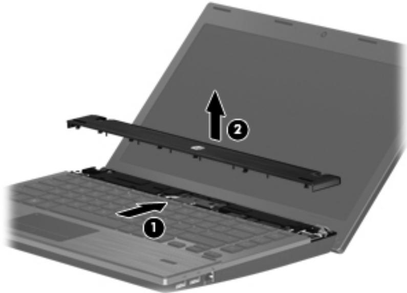
Reverse this procedure to install the switch cover and keyboard.
