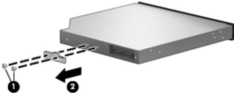
Reverse this procedure to reassemble and install an optical drive.
