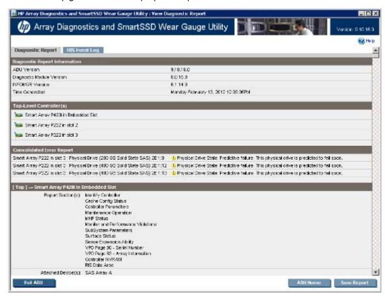
The diagnostic report includes an additional RIS Event Log tab. Smart Array controllers store configuration data in the RAID information sector of all physical drives. The RIS Event Log reads the data and displays the decoded change logs.
