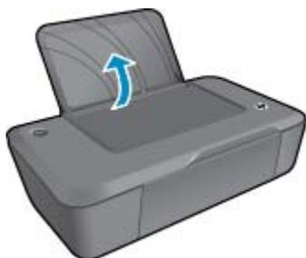
2. Lower the output tray and pull out the tray extender.
