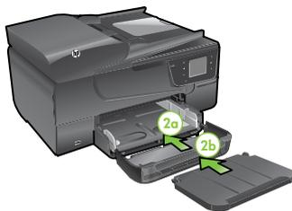
Install the input tray and the output tray.
