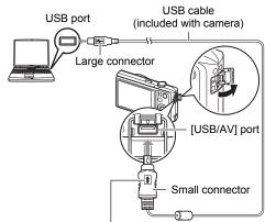
Making sure that the 1 mark on the USB cable connector is towards the lens side, connect the cable to the camera.
