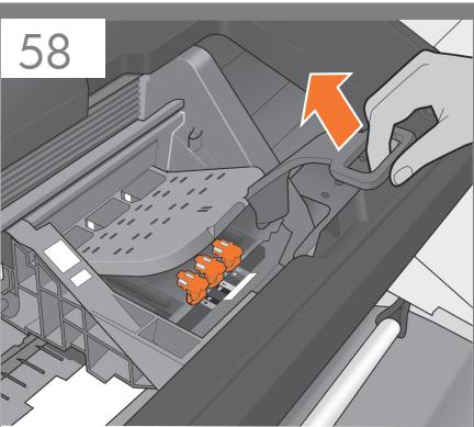
EN Lift the handle up to open the printhead cover. The front panel prompts you for the next step: removing the printheads. Do not press OK until you have removed all the orange setup printheads.
