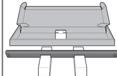
Place the two pieces of packaging material on the floor, spaced 40 cm apart, and place the cross-brace on top of them.
