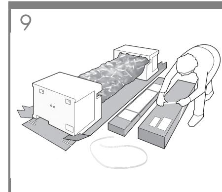
Cut and remove the straps around the stand box.
