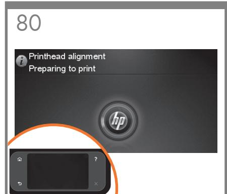
The product will proceed to align the print-heads. This process involves printing, and therefore needs to use paper with a straight leading edge. **Note:** printhead alignment requires paper at least 24in (61cm) wide. Roll paper is recommended.
