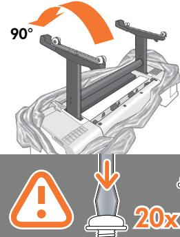
Rotate the product 90 degrees. **IMPORTANT:** make sure that the roll feeds are facing downwards.
