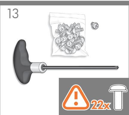
**EN** A screwdriver and 22 screws are provided in the stand box: 16 screws to assemble the stand, 4 to attach it to the product, and **2 are spare**. Do not try to remove the washers from the screws. **Note:** All the screws are for the stand. The basket does not need screws.
