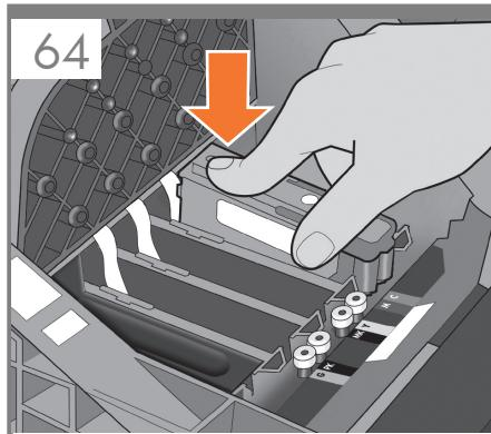
Push each printhead into the slot until it clicks into place. The front panel tells you whether the printhead has been inserted correctly.
