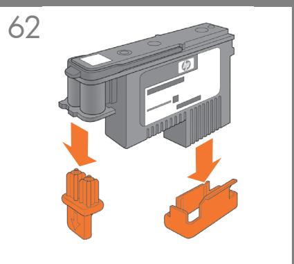
**EN** Unwrap each printhead and remove all orange parts.
