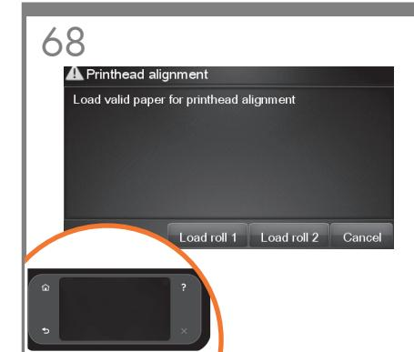
Once the printhead check has finished the product will be ready to load paper for the printhead alignment.
