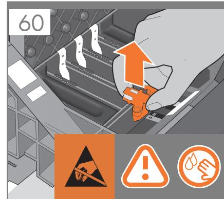
EN Remove and discard all orange setup printheads. You may need to use force to extract each printhead. The setup printheads contain ink, which could leak out. Avoid touching pins, leads or circuits.
