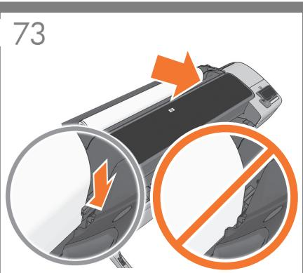
**EN** Feed the leading edge of the paper into the product until the product takes hold of it. Do not insert the roll paper into the cutsheet slot. **Note:** do not close the roll cover until the front panel notifies you.
