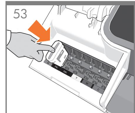
Insert the ink cartridges one by one. Each cartridge is marked with its own color, and should be inserted only into the slot of the same color. Avoid touching pins, leads or circuits.
