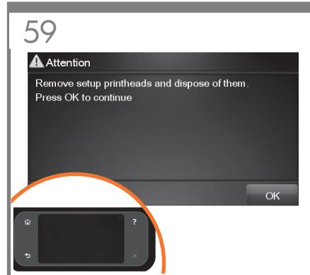
The setup printheads exist only to prevent the escape of ink during ink cartridge installation. The front panel now prompts you to remove the setup printheads and press the OK key when you have finished.
