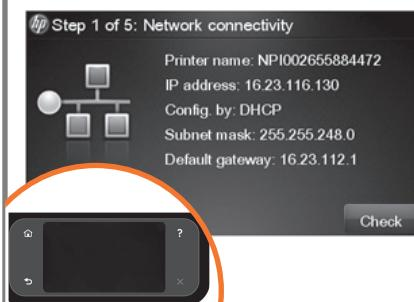
The connectivity wizard will help you configure your LAN and Internet connection, verify the automatic Firmware upgrade configuration, and also help you with the ePrint & Share configuration so that you have its settings enabled, such as remote printing and eprint.
