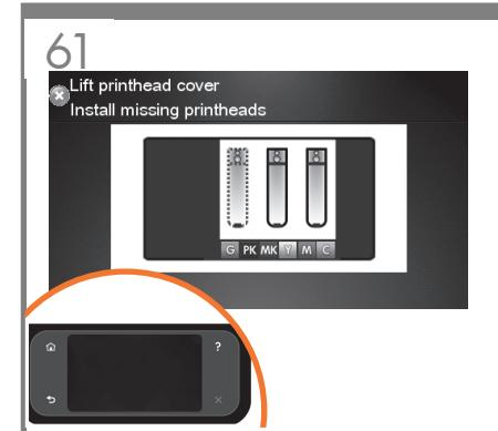
EN Press the OK key on the front panel when you have removed all of the setup printheads. The front panel then prompts you to install the new printheads.
