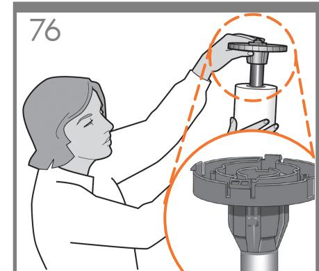
**Only for T1300:** If the blue removable stop is on the spindle, remove it. Put the roll onto the spindle, making sure to put it on the right way round: the leading edge of the paper should go into the product from the top of the roll. Add the removable stop to the spindle to keep the roll in place.
