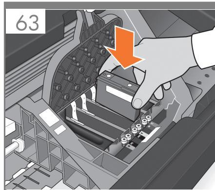
Insert the prinheads one by one. Each printhead is marked with its own colors, and should be inserted only into the correct slot marked with the same colors. Insert the prinheads with the blue handle towards you.
