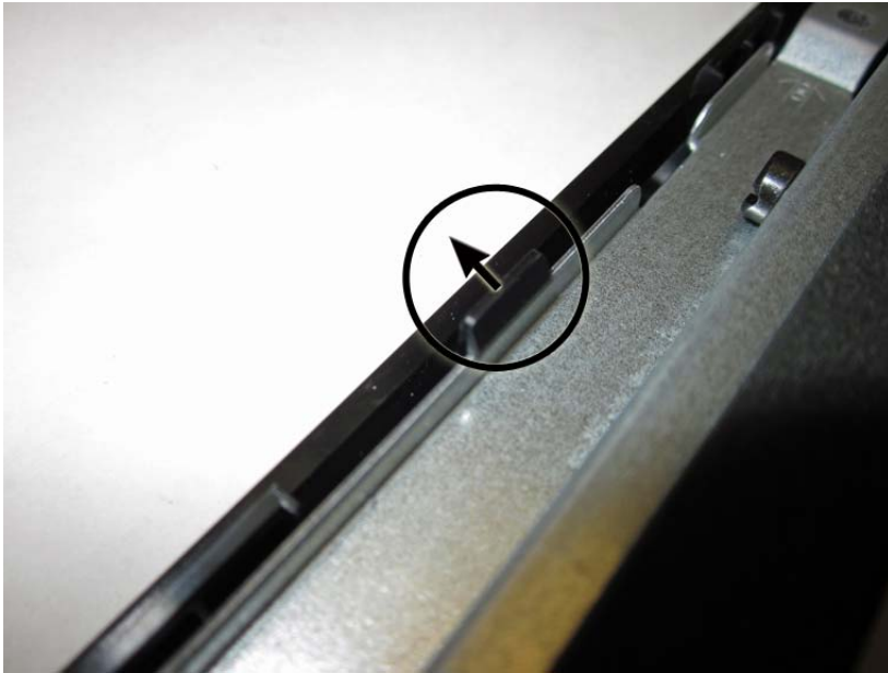
Figure 7-32 Removing the bezel from the display assembly
