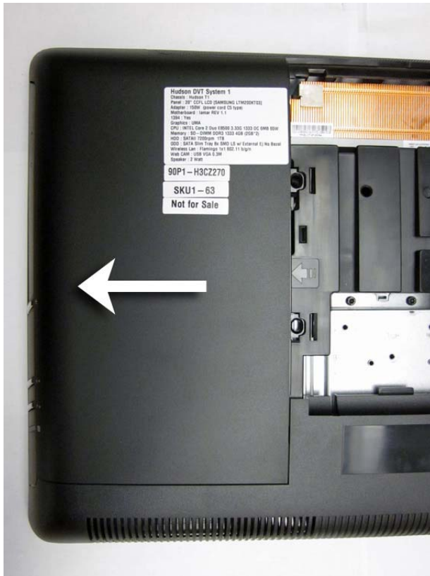
Figure 7-3 Removing the left rear cover
