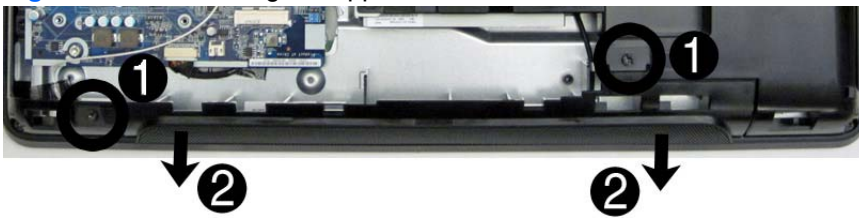
Figure 7-19 Removing the upper cover
