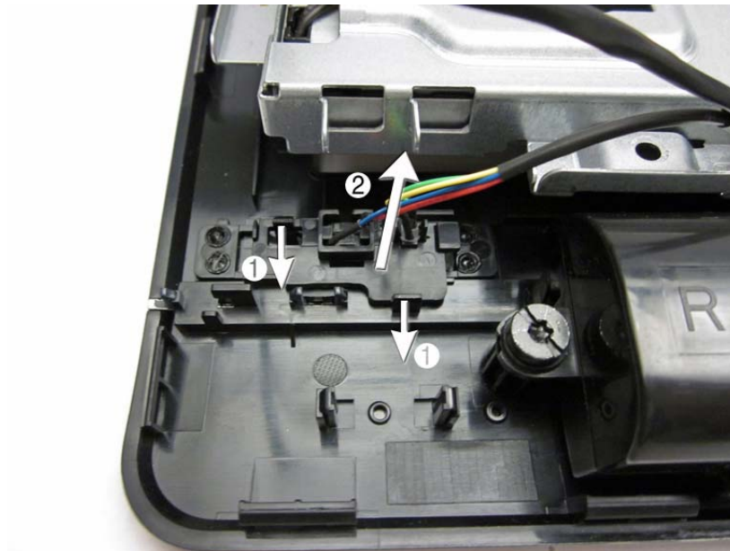
Figure 7-31 Removing the power button assembly from the bezel
