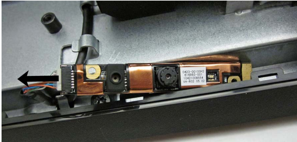
Figure 7-18 Disconnecting the webcam module cable
