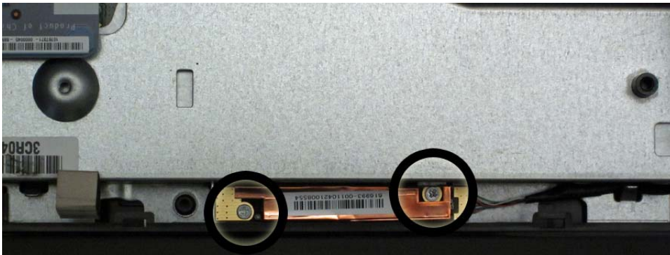
Figure 7-17 Removing the webcam module screws
