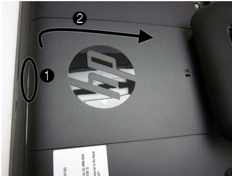
Figure 7-1 Removing the small rear cover
