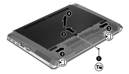
Reverse the removal procedures to install the bottom door.
