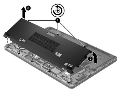
5. If you are replacing a memory module, remove the existing memory module:
