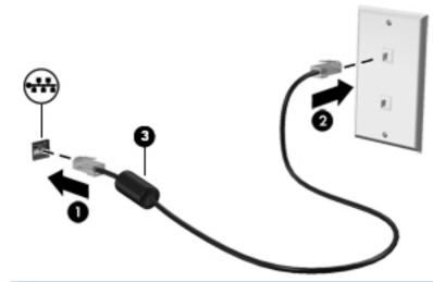
**WARNING!** To reduce the risk of electric shock, fire, or damage to the equipment, do not plug a modem or telephone cable into the RJ-45 (network) jack.
