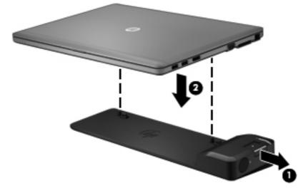
3. Push in the connect button (1) on the docking device to secure the docking device to the computer. The connect light (2) turns on when the computer is fully docked.
