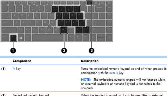
NOTE: The embedded numeric keypad will not function while an external keyboard or numeric keypad is connected to the computer.
