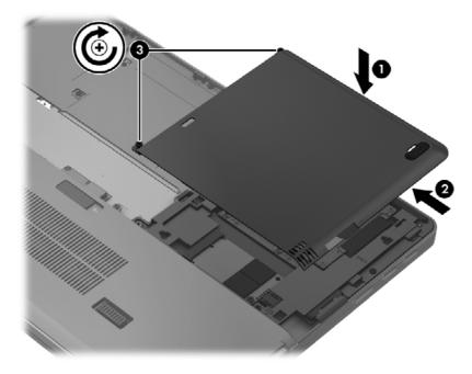
3. Insert the battery (see <u>Inserting or removing the battery on page 31</u>).
