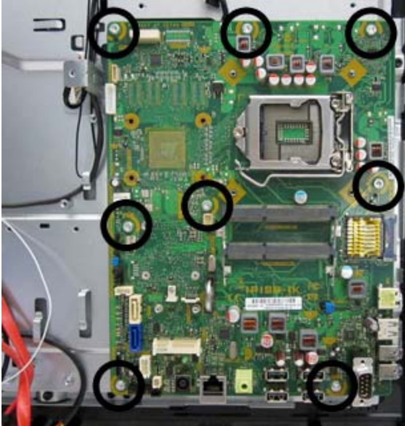
Figure 6-63 System board screw locations
