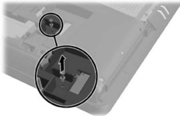
Figure 6-10 Removing the optical disc drive security screw
