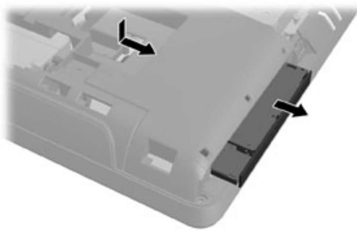
Figure 6-11 Removing the optical disc drive
