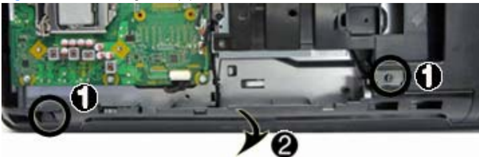
Figure 6-37 Removing the top panel
