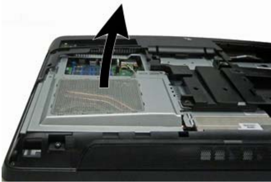
Figure 6-30 Removing the heat sink cover
