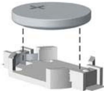
Figure 6-25 Removing a coin cell battery (Type 1)
