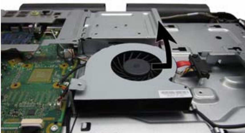
Figure 6-45 Removing the fan
