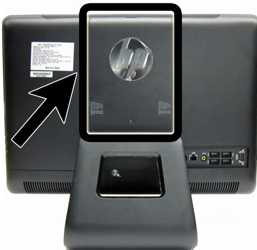
Figure 6-1 Hinge cover panel location
