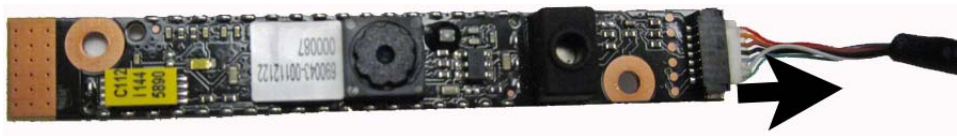
Figure 6-40 Disconnecting the webcam module
