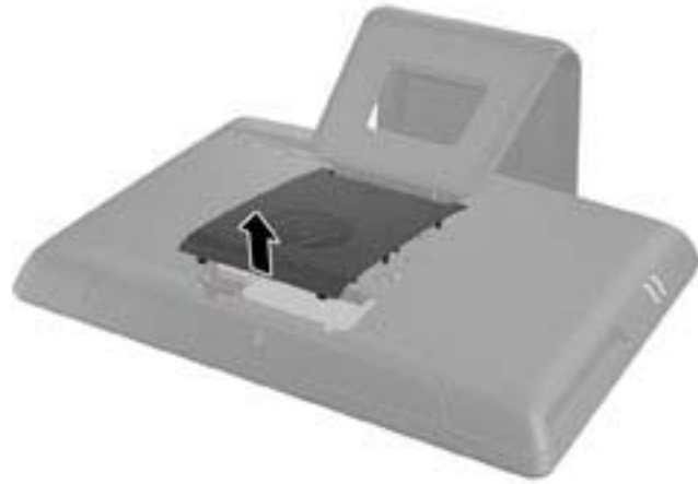
Figure 6-2 Removing the hinge cover panel
