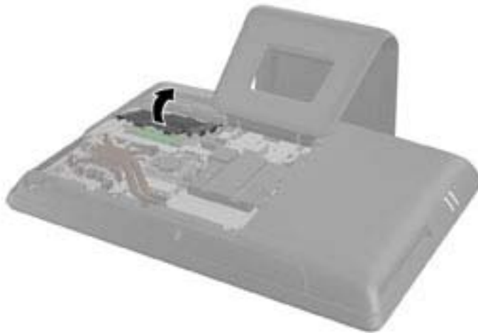
Figure 6-24 Removing the memory cover
