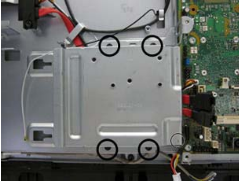
Figure 6-60 Stand bracket screw locations
