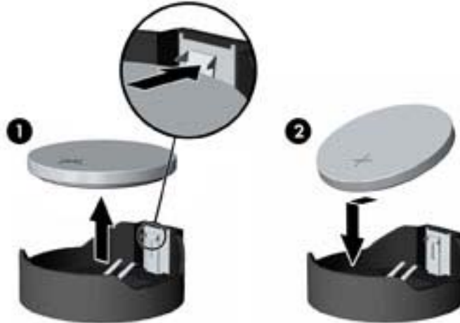
Figure 6-26 Removing and replacing a coin cell battery (Type 2)
