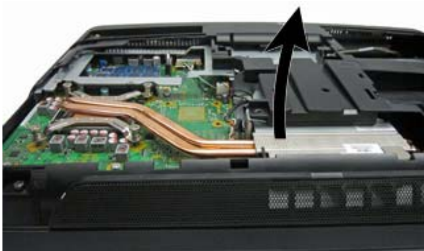
Figure 6-34 Removing the heat sink
