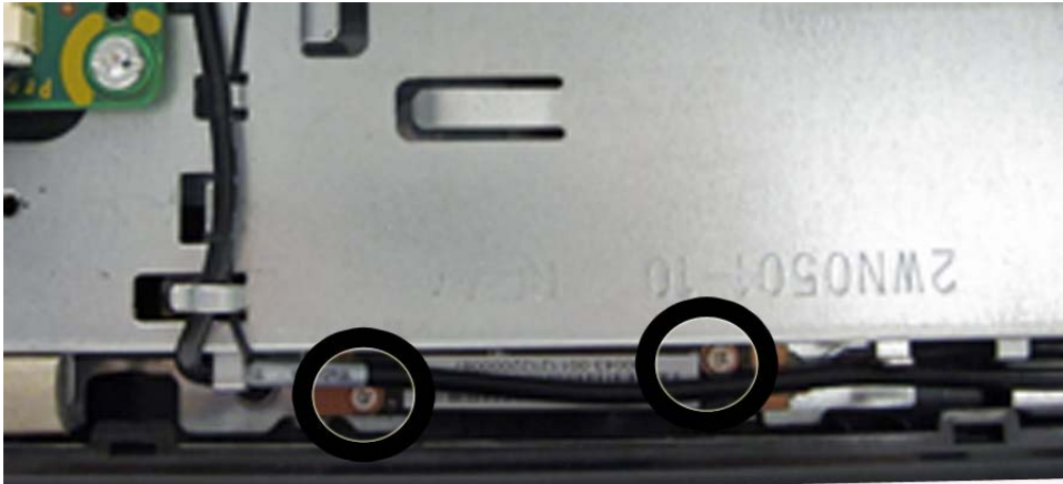
Figure 6-39 Webcam module screws
