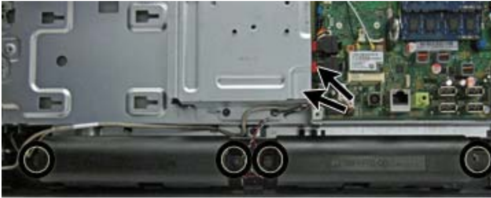
Figure 6-58 Removing the speakers
