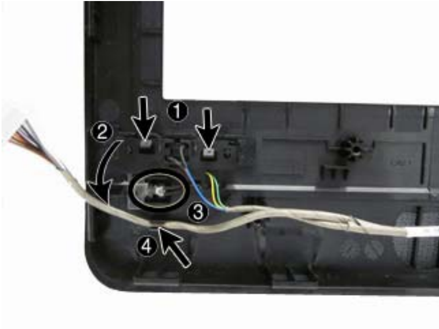
Figure 6-73 Removing the power switch assembly
