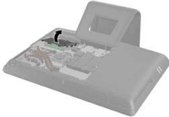
Figure 6-19 Removing the memory cover
