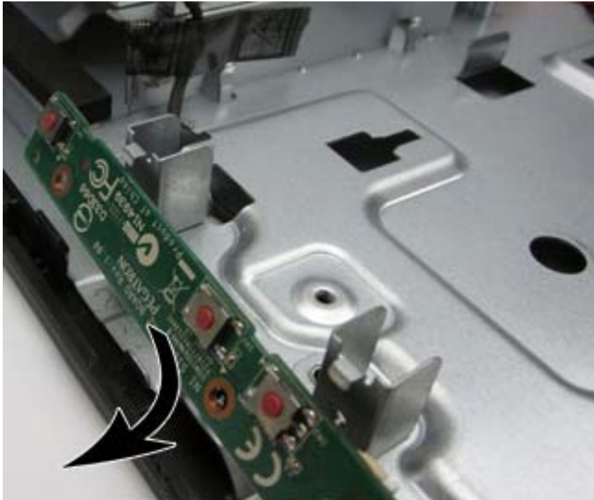
Figure 6-51 Removing the sidekey board
