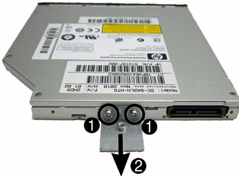
Figure 6-12 Removing the optical drive bracket
