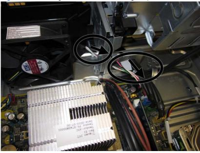
To install the front I/O and power switch assembly, reverse the removal procedure.
