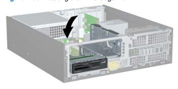
7. If installing a media card reader, connect the USB cable from the media card reader to the USB connector on the system board labeled MEDIA1.
