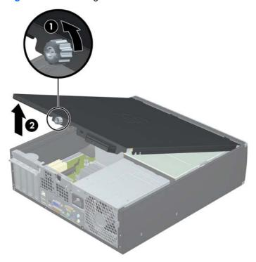
To install the access panel, reverse the removal procedure.
