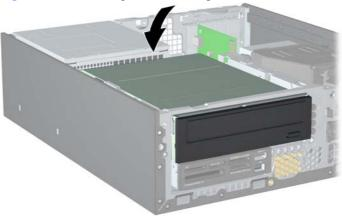
6. Slide the drive back until it stops, then lift it up and out of the drive cage.
