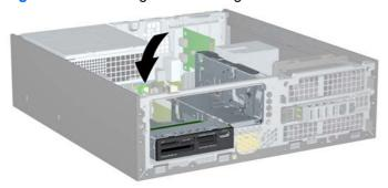
5. Slide the drive back until it stops, then lift it up and out of the drive cage.
