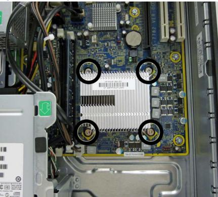
**6.** Lift the heat sink from atop the processor and set it on its side to keep from contaminating the work area with thermal grease.
