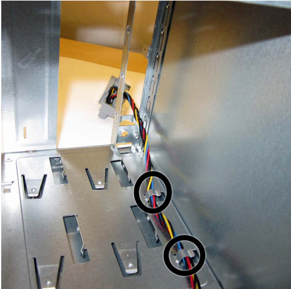
Figure 7-39 Power switch cable routing
