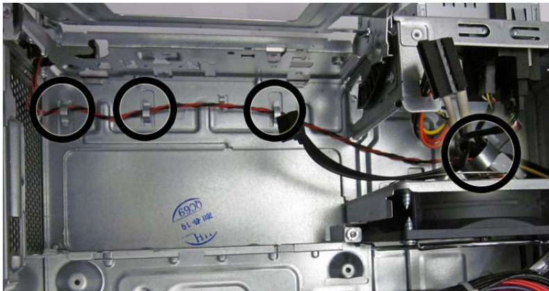
Figure 8-23 Removing the power switch cable
