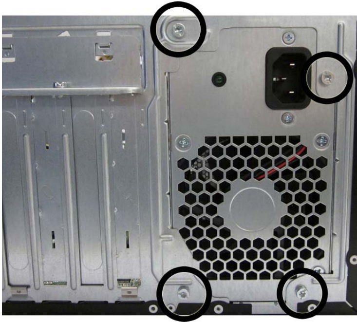
Figure 7-48 Power supply screws
