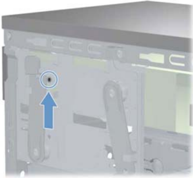
Figure 7-28 Optical drive alignment hole
