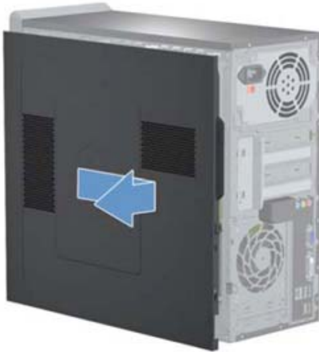
Figure 7-2 Removing the access panel
