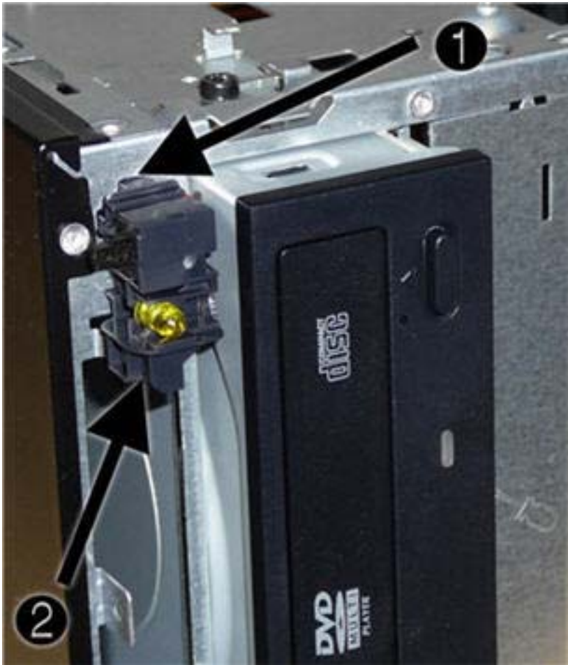
Figure 7-40 Removing the power switch assembly
