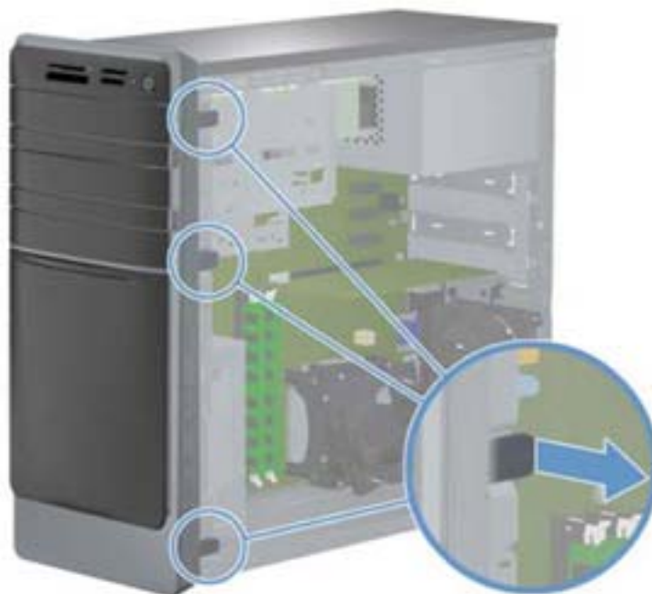
Figure 7-3 Removing the Front Bezel
