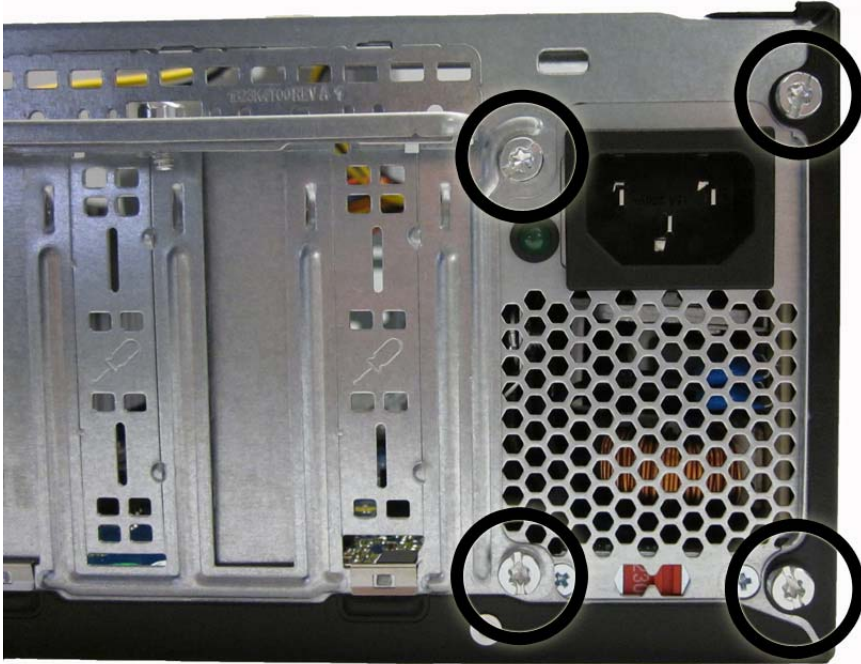
Figure 8-36 Removing the power supply screws
