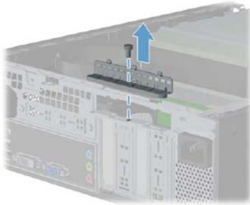
Figure 8-10 Opening the expansion slot bracket
