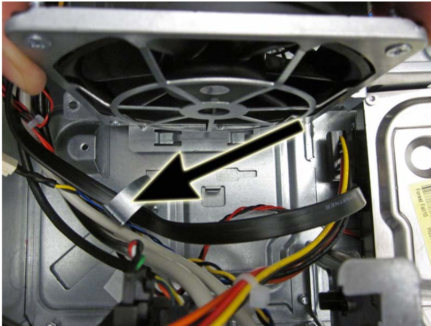
Figure 8-26 Removing the cables from the clip
