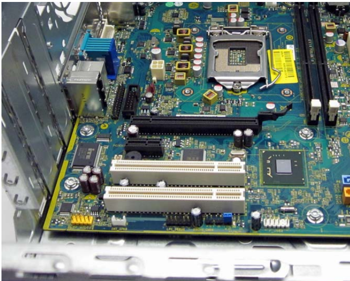
Figure 7-17 Expansion slot locations (HP Pro 3330/3380 shown)
