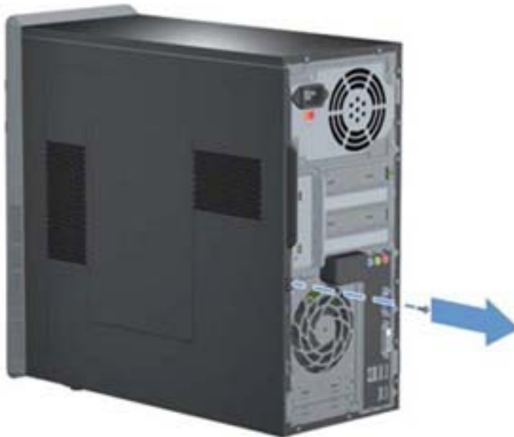
Figure 7-1 Removing the access panel screw
