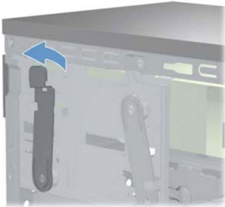
Figure 7-24 Pushing the optical drive
