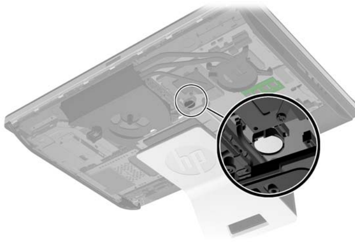
Figure 2-24 Locating the Battery
