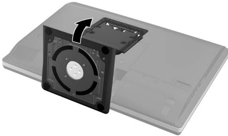
Figure 2-14 VESA Mounting Holes
