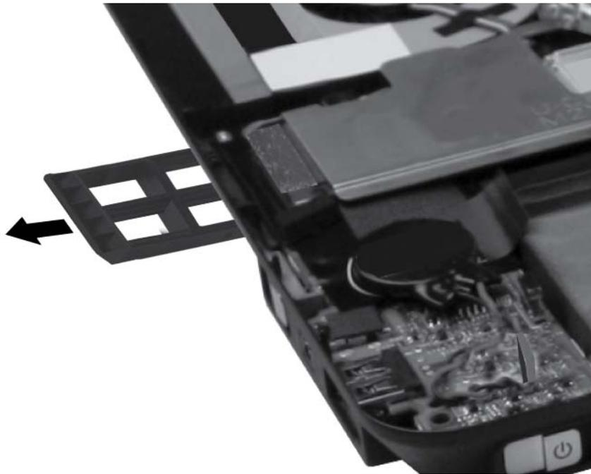
3. Peel back the adhesive strip **(2)** on the system board to reveal one of the two screws required to remove the system board.
