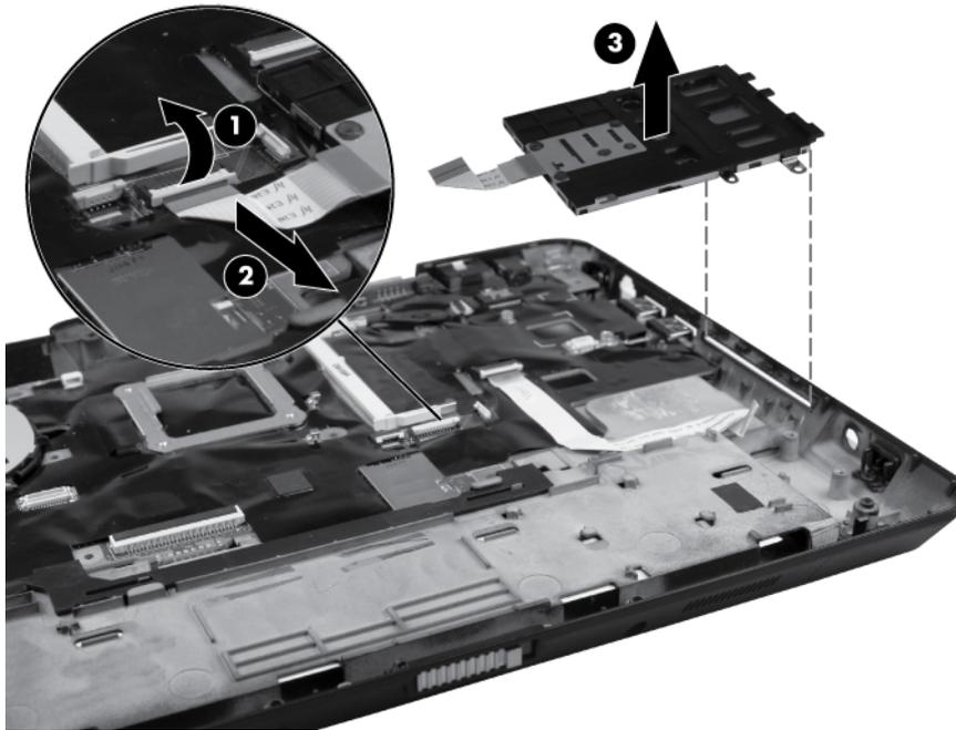
4. Remove the Bluetooth cable by disconnecting the ZIF cable (1) securing the Bluetooth module to the system board and then lift the cable (2).
