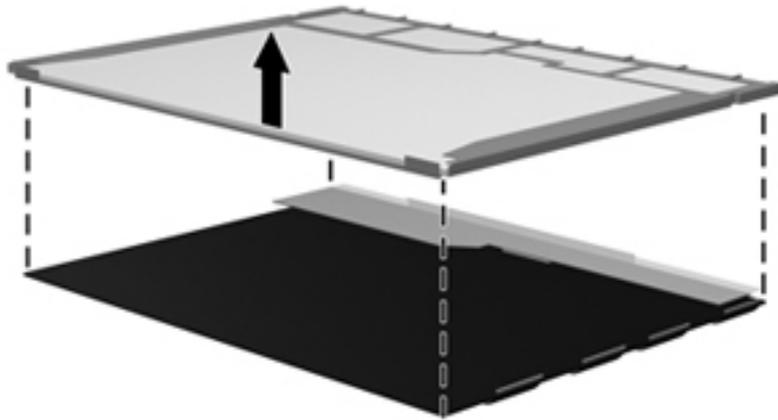
**24.** Recycle the LCD panel and backlight.
