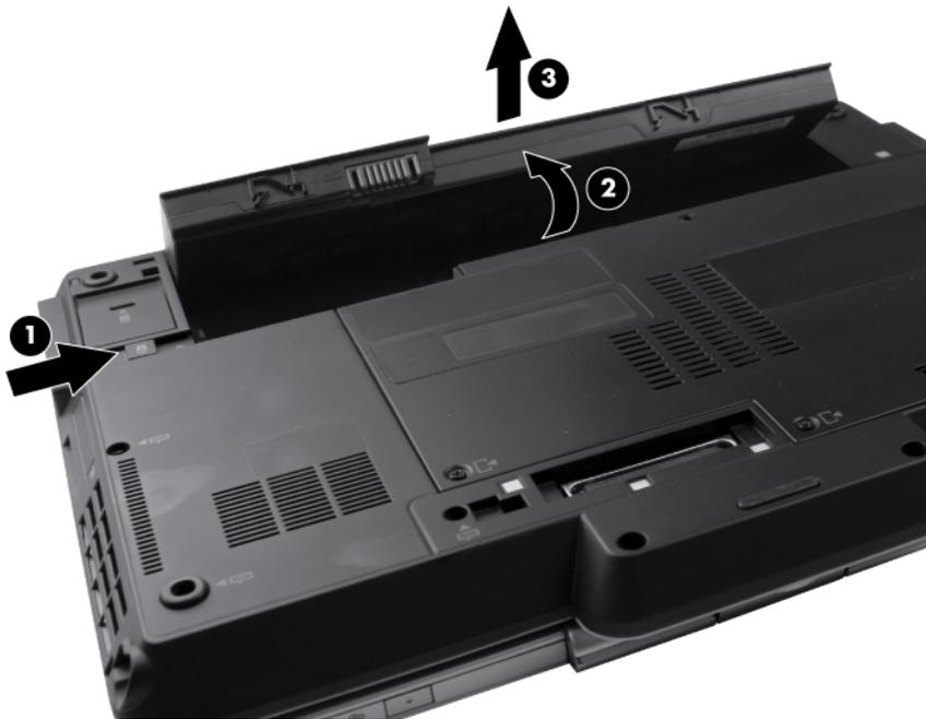
To insert the battery, insert the front edge of the battery into the battery bay and pivot the rear edge of the battery downward until it is seated. The battery release latch automatically locks the battery into place.
