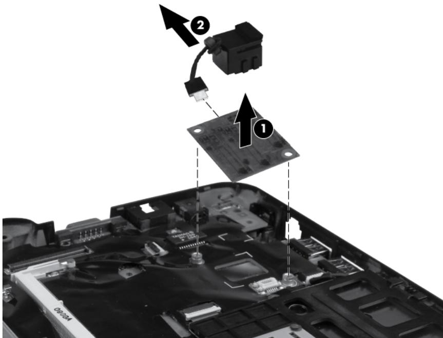
Reverse this procedure to install the modem module.
