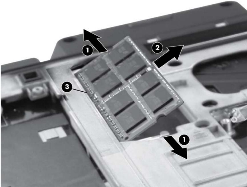
Reverse this procedure to install a primary memory module.
