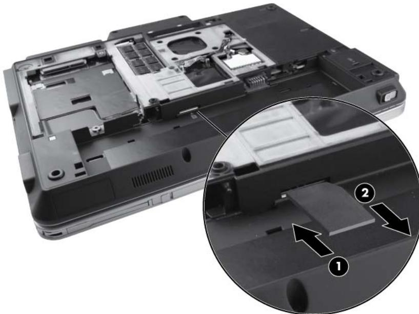
Reverse this procedure to install the SIM.
