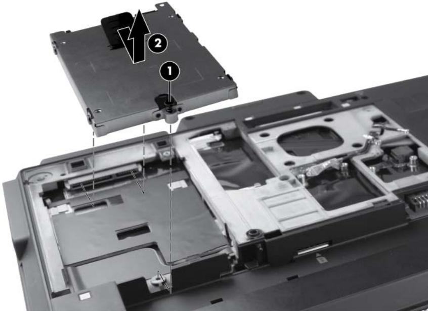
4. If it is necessary to replace the hard drive bracket, remove the four Phillips M2.5x3.0 screws **(1)** that secure the bracket to the hard drive.
