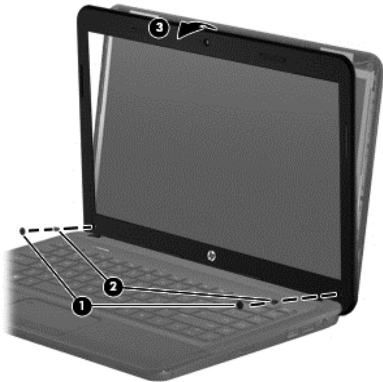
5. To remove the webcam/microphone module:
