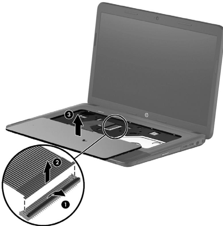
Reverse this procedure to install the keyboard.
