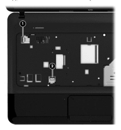
7. Remove the two Phillips PM2.5×6.0 screws that secure the top cover to the computer.
