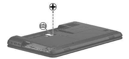
2. Rest and secure the computer on its left side with the bottom toward you, and then partially open the computer.
