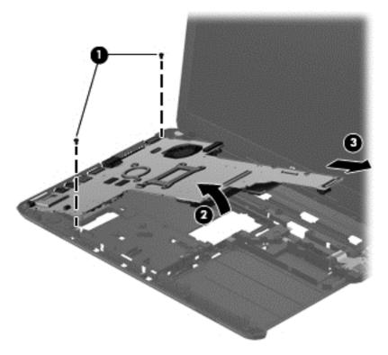
NOTE: A thermal pad services a component on the bottom of the system board. Replacement thermal material is included with all system board spare part kits.
