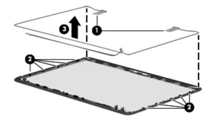
6. If replacing the display enclosure, be sure that the other subcomponents (including the webcam/ microphone module, the antenna receivers, and all associated cables and hardware) are transferred to the new enclosure.
