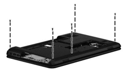
3. Remove the four Phillips PM1.6×2.0 screws (1) and the Phillips PM2.0×3.0 screw (2) that secure the top cover to the computer.
