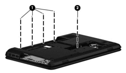
4. Remove the eleven Phillips PM2.5×4.0 screws that secure the top cover to the computer.
