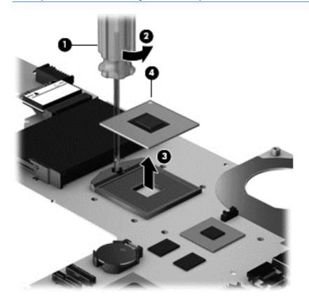
Reverse this procedure to install the processor.
