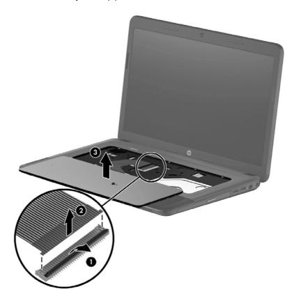
Reverse this procedure to install the keyboard.
