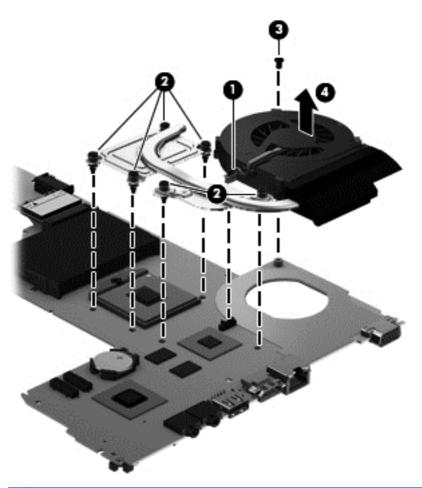
NOTE: The following illustration shows the fan/heat sink assembly removal process on a computer model equipped with an Intel processor and a graphics subsystem with UMA memory.
