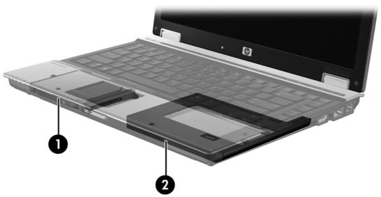
The following illustration shows a supported computer with the primary hard drive (1) and secondary hard drive (2), with the third drive in the Upgrade Bay (3) that allows RAID 5.
