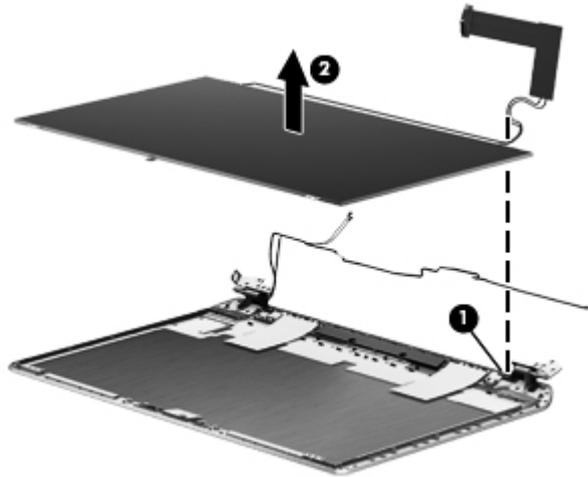
9. If it is necessary to replace the display panel cable:
