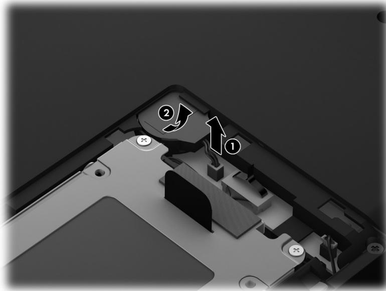
3. Remove the RTC battery.
