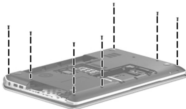
2. Remove the three Phillips PM2.5×5.5 screws that secure the top cover to the computer.
