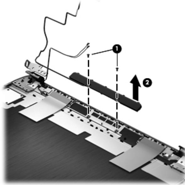
**13.** If it is necessary to replace the wireless antenna cables and transceivers:
