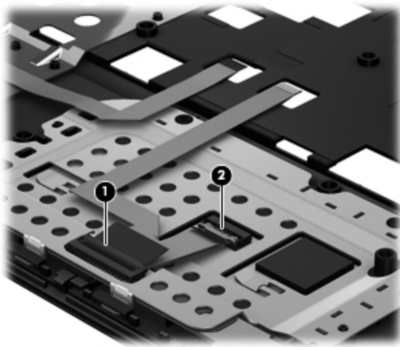
4. Remove the two Phillips PM2.5x3.5 screws **(1)** that secure the TouchPad button board bracket to the top cover.
