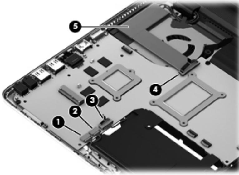
9. Disconnect the USB board cable **(1)** from the system board.
