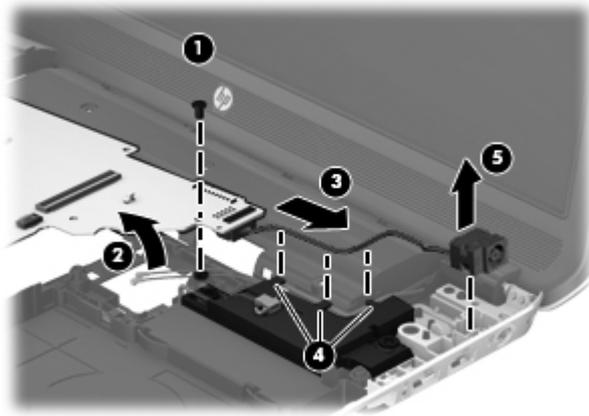
5. Remove the power connector cable.
