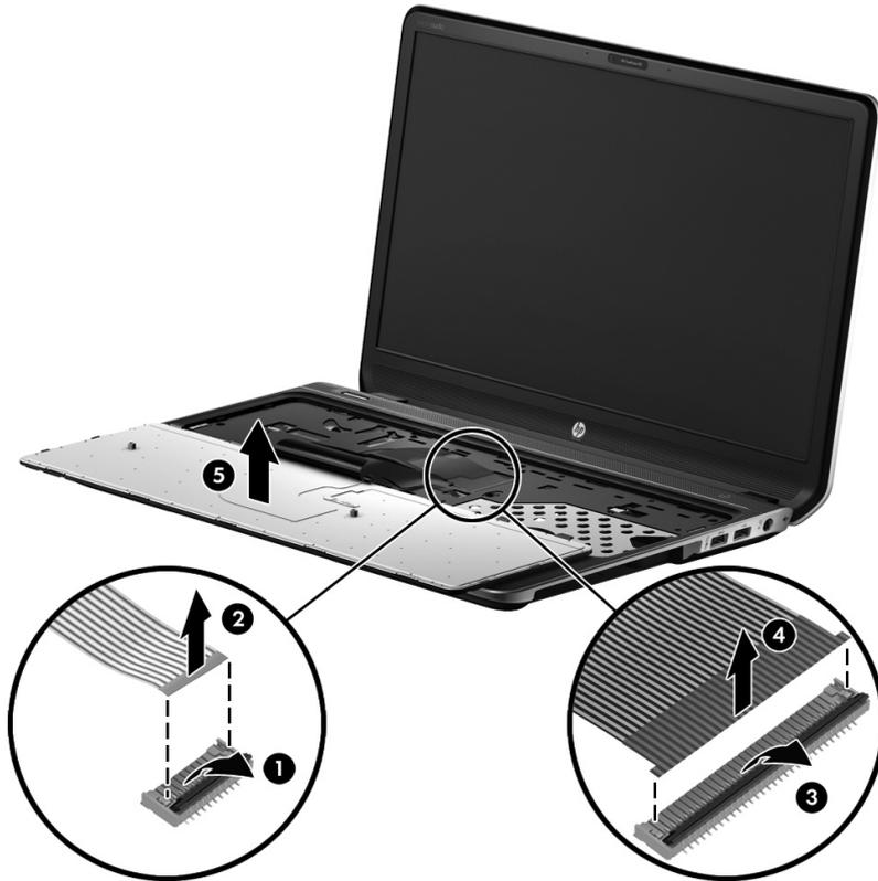
Reverse this procedure to install the keyboard.
