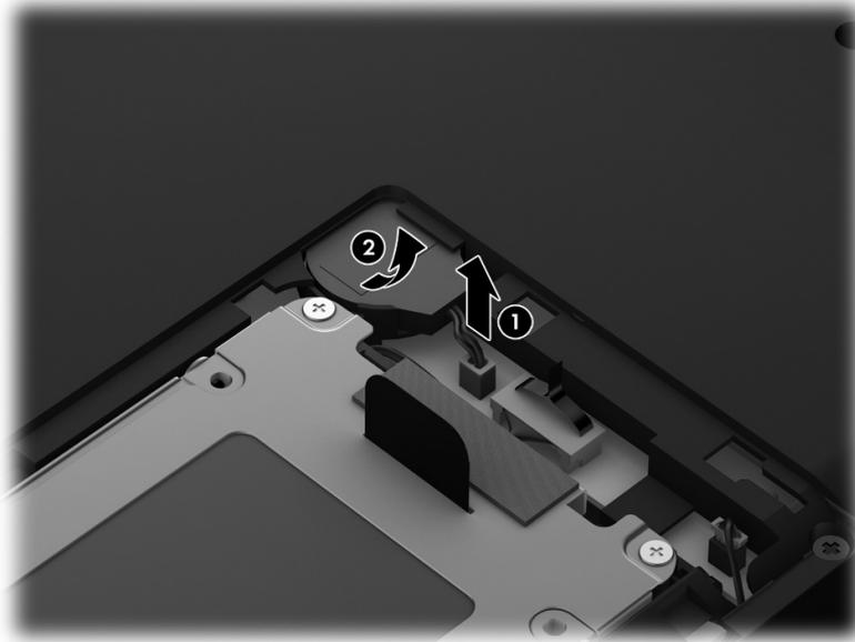
3. Remove the RTC battery.
