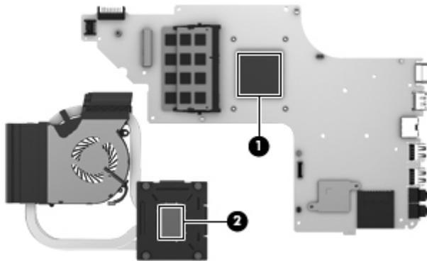
**NOTE:** The following illustration shows the replacement thermal material locations on a computer model equipped with an Intel processor and a graphics subsystem with discrete memory.
