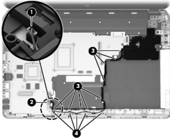
4. Remove the two Phillips PM2.5×10.0 screws **(1)** that secure the subwoofer to the base enclosure.
