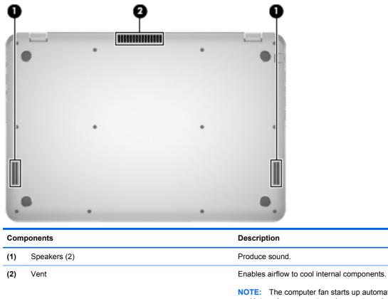
**NOTE:** The computer fan starts up automatically to cool internal components and prevent overheating. It is normal for the internal fan to cycle on and off during routine operation.
