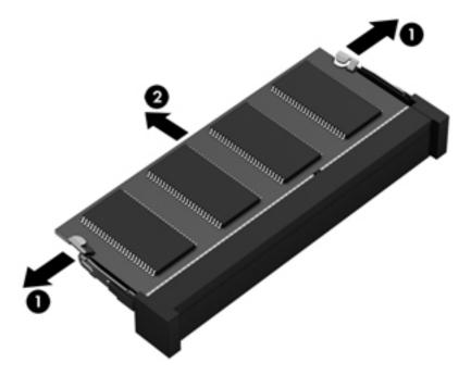
Reverse this procedure to install the memory module.
