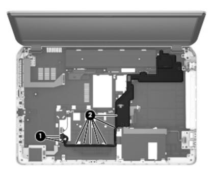
2. Remove the two Phillips PM2.5×10.0 screws (1) that secure the subwoofer to the base enclosure.
