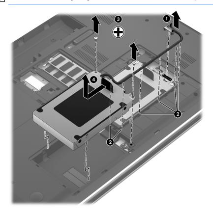
11. If it is necessary to replace the hard drive screws (1), hard drive bracket (2), or hard drive connector cable (3), remove and replace the components. The hard drive screws, hard drive bracket, primary hard drive connector cable, and secondary hard drive connector cable are available in the Hard Drive Hardware Kit, spare part number 681976-001.
