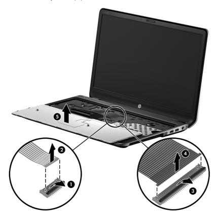
Reverse this procedure to install the keyboard.
