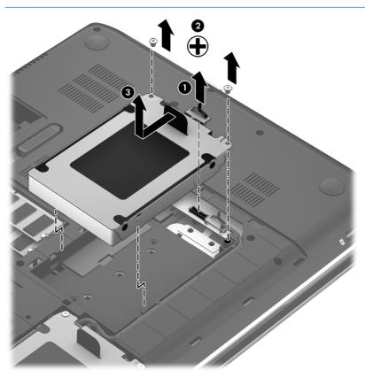
7. Disconnect the secondary hard drive connector cable (1) from the system board.
