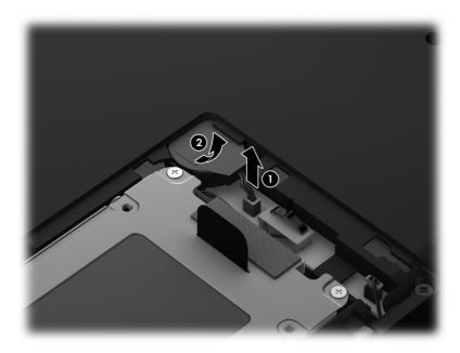
3. Remove the RTC battery.
