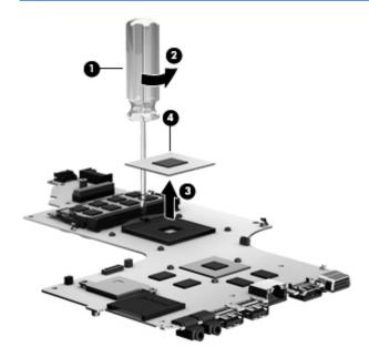
Reverse this procedure to install the processor.
