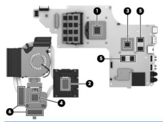
NOTE: The following illustration shows the replacement thermal material locations on a computer model equipped with an Intel processor and a graphics subsystem with UMA memory. Thermal paste is used on the processor (1) and the heat sink section (2) that services it.
