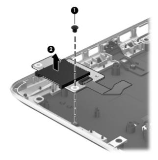
Reverse this procedure to install the Card Reader board.
