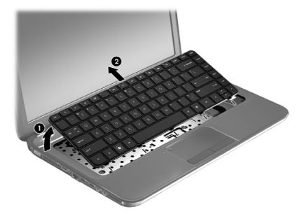
7. Tilt the keyboard forward (1) onto the palm rest. Release the zero insertion force (ZIF) connector (2) to which the keyboard cable is attached, and then disconnect the keyboard cable (3) from the system board.
