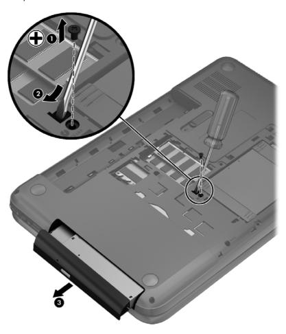
**4.** Remove the two Phillips M2.0 x 3.0 screws **(1)** that secure the optical drive bracket to the optical drive and then remove the bracket **(2)** from the optical drive.
