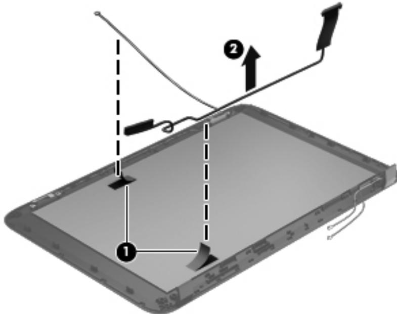
11. If it is necessary to replace the wireless antenna cables and transceivers:
