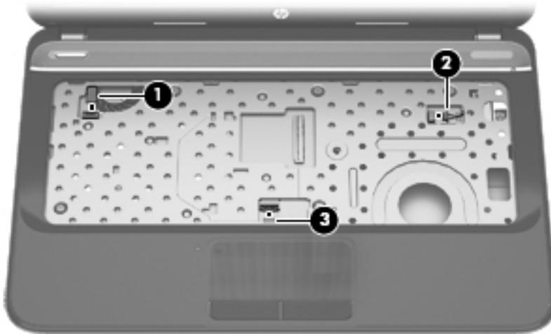
2. Remove the following screws under the keyboard:
