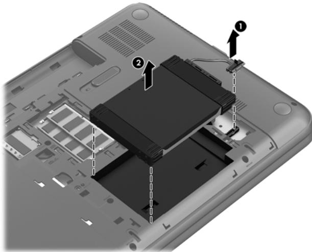
3. Disconnect the hard drive cable **(1)**. Remove the front bumper **(2)** and back bumper **(3)**.
