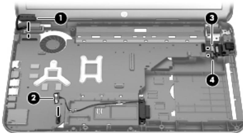
2. Remove the Phillips M2.5 × 4.5 screw **(1)** that secures the system board to the base enclosure.
