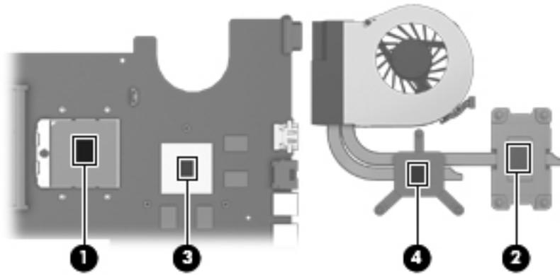
1. If it is necessary to replace the fan, turn the fan and heat sink upside down with the fan toward you.
