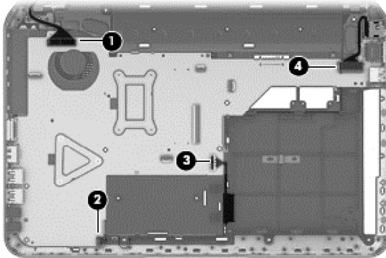
2. Remove the three Phillips PM2.0×5.5 screws (1) that secure the system board to the base enclosure.
