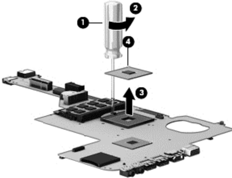
Reverse this procedure to install the processor.
