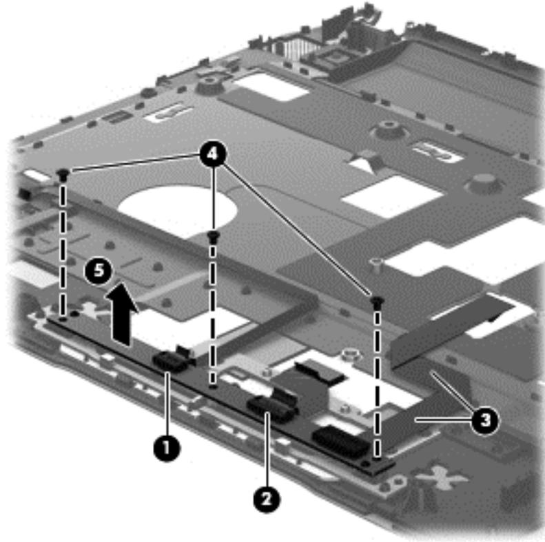
Reverse this procedure to install the TouchPad button board and cable.
