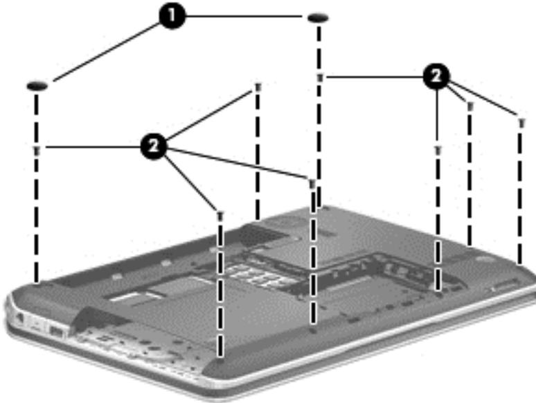
3. Remove the Phillips PM2.0×2.0 screws in the optical drive bay (1) and the hard drive bay (2).
