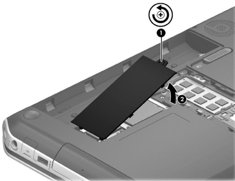
3. Remove the wireless module compartment cover.
