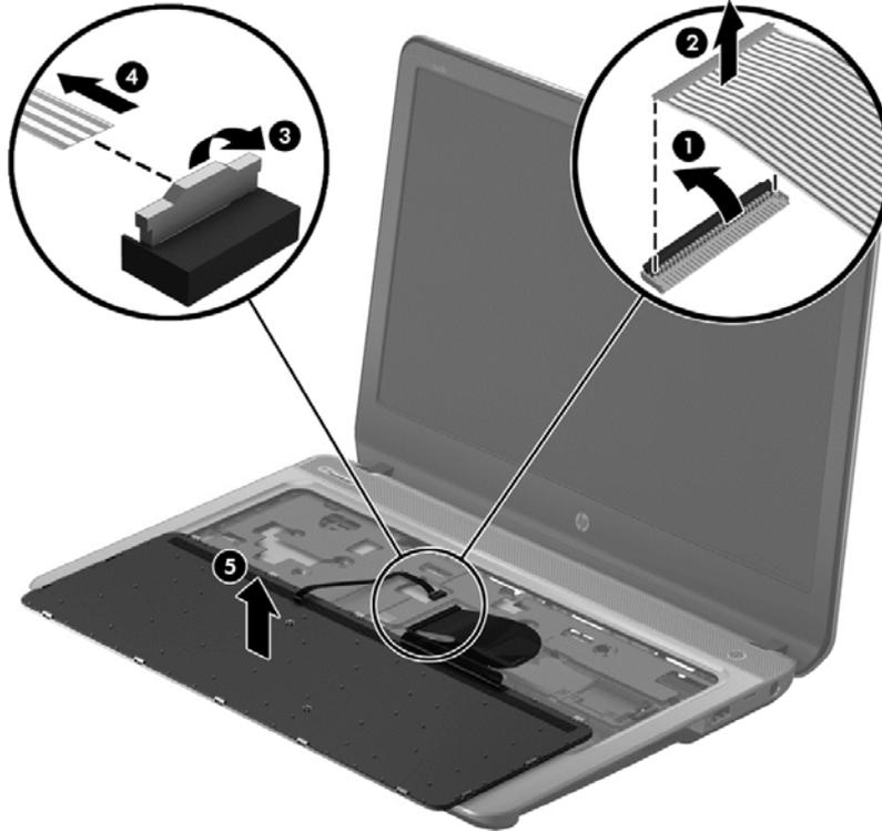
Reverse this procedure to install the keyboard.
