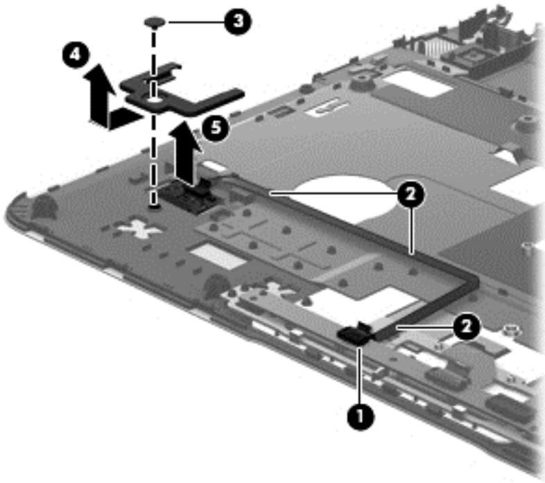
Reverse this procedure to install the fingerprint reader board.
