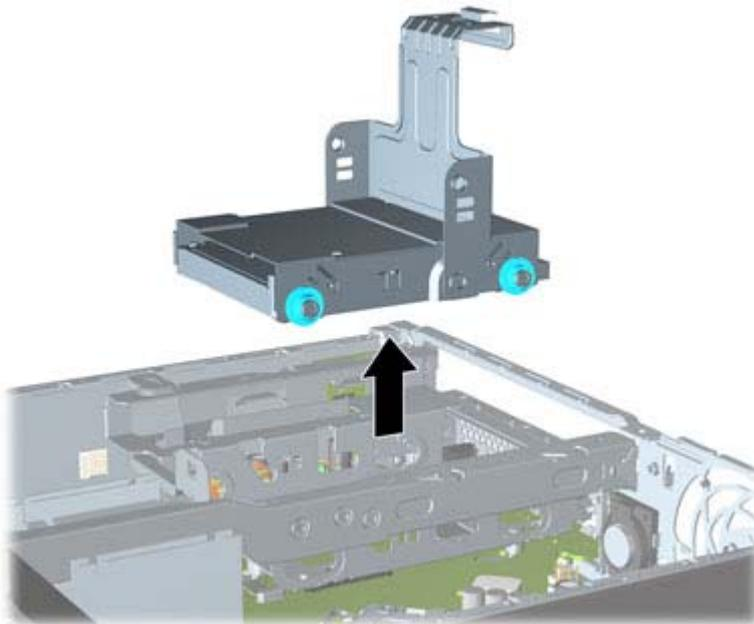
6. Remove the four guide screws from the sides of the hard drive carrier.
