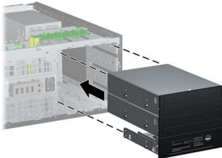
**CAUTION:** The bottom 5.25-inch drive bay has a shorter depth than the upper two bays. The bottom bay supports a half-height drive or other device that is no more than 14.5 cm (5.7 inches) in depth. Do not try to force a larger drive, such as an optical drive, into the bottom bay. This could cause damage to the drive and the system board. The use of unnecessary force when installing any drive into the drive bay may result in damage to the drive.
