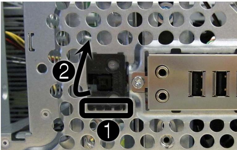
7. Pull the assembly away from the chassis while threading the cable through the hole in front of the chassis.
