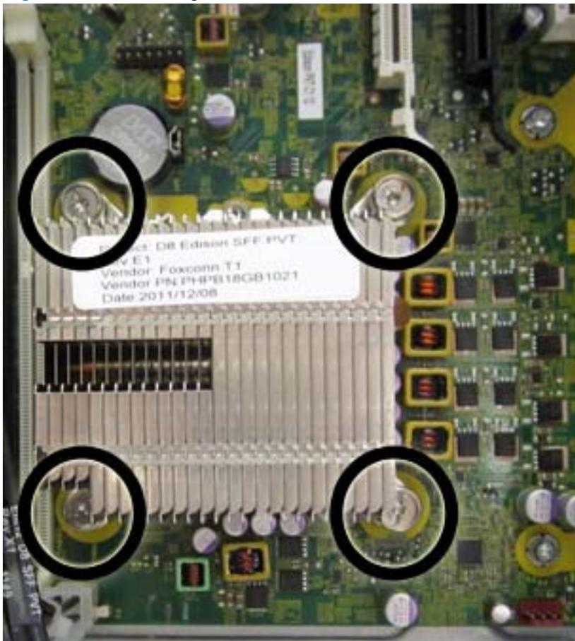
5. Lift the heat sink from atop the processor.
