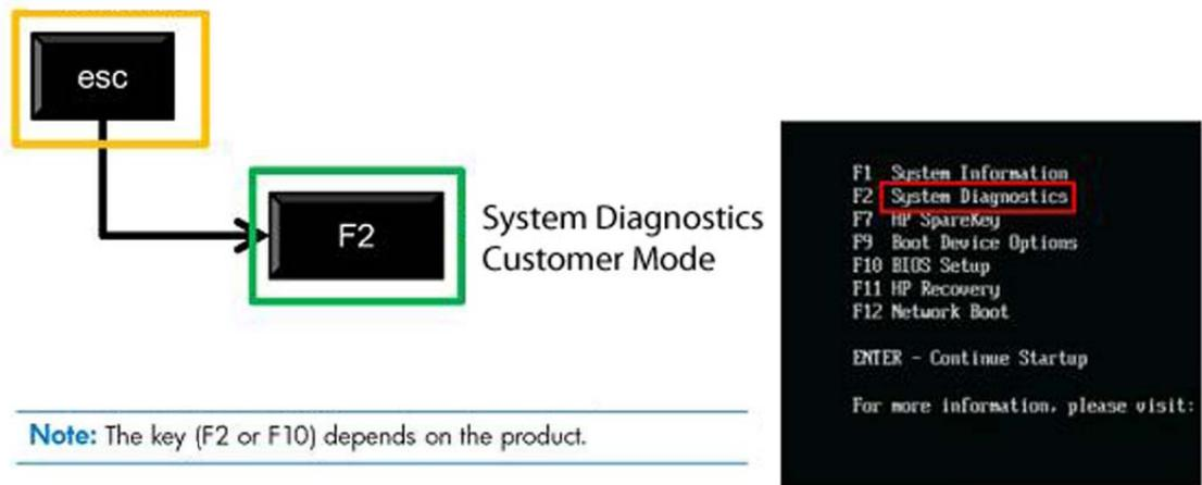
After pressing **F2**, the BIOS sequentially searches three places for the system diagnostics:
