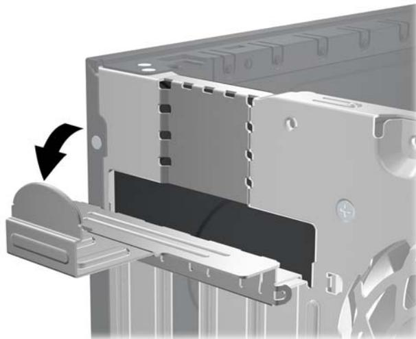
5. Before installing an expansion card, remove the expansion slot cover or the existing expansion card.
