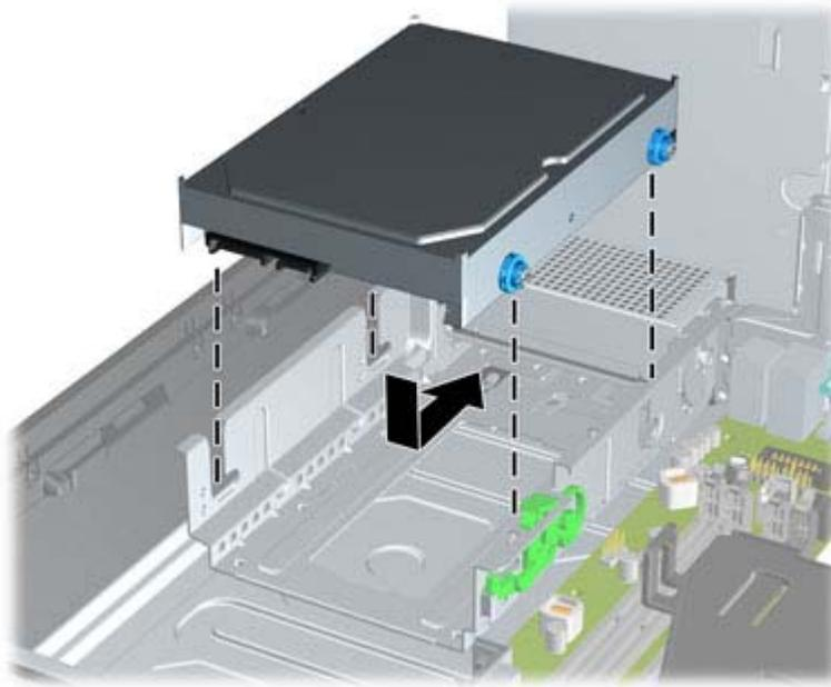
9. Connect the power cable and data cable to the back of the hard drive.
