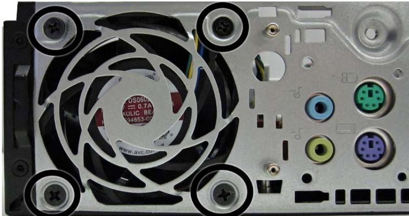
10. From the inside of the chassis, slide the fan out from underneath the chassis lip, and then remove the fan.
