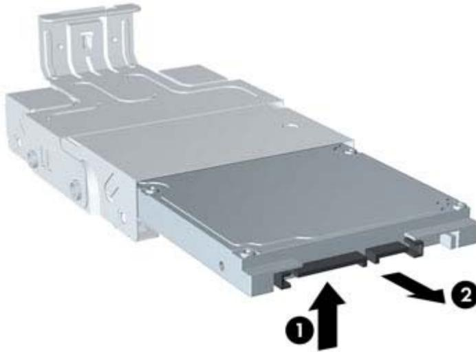
8. Position the hard drive so that the top of the hard drive is up against the top of the carrier (1) so that the circuit board on the bottom of the hard drive does not come in contact with the tabs on the bottom of the carrier, then slide the new hard drive into the carrier (2).
