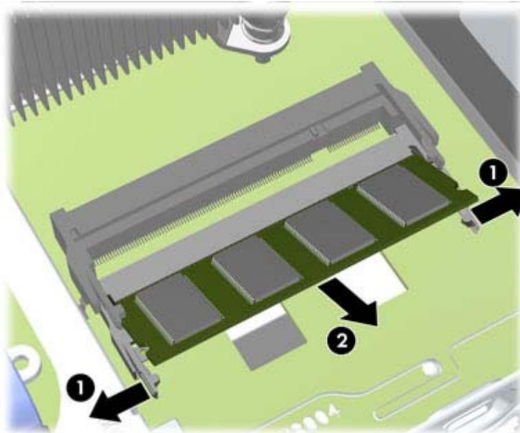
5. Slide the new SODIMM into the socket at approximately a 30° angle (1) then press the SODIMM down (2) so that the latches lock it in place.
