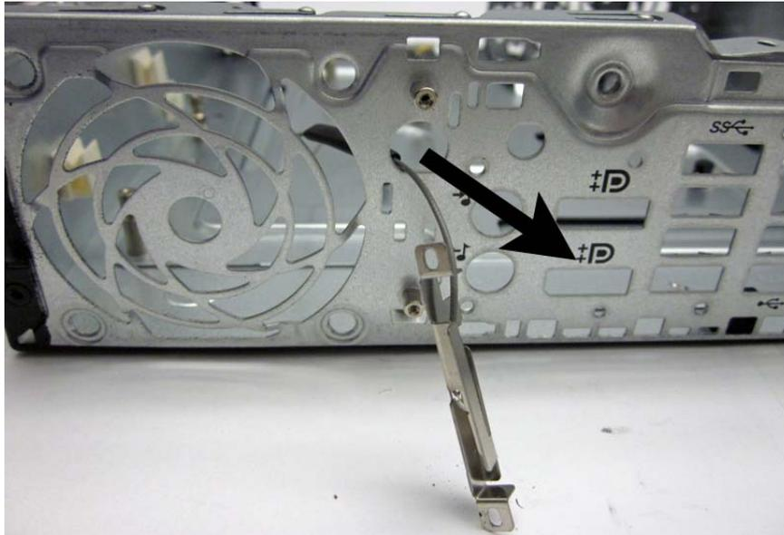
To install the rear fan, reverse the removal procedure.
