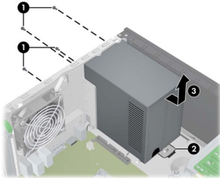
To install the power supply, reverse the removal procedure.
