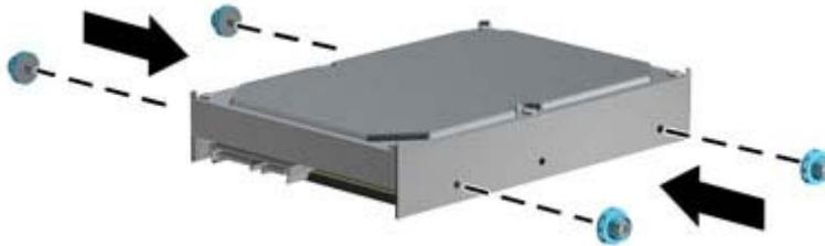
8. Align the guide screws with the slots on the chassis drive cage, press the hard drive down into the bay, then slide it back until it stops and locks in place.
