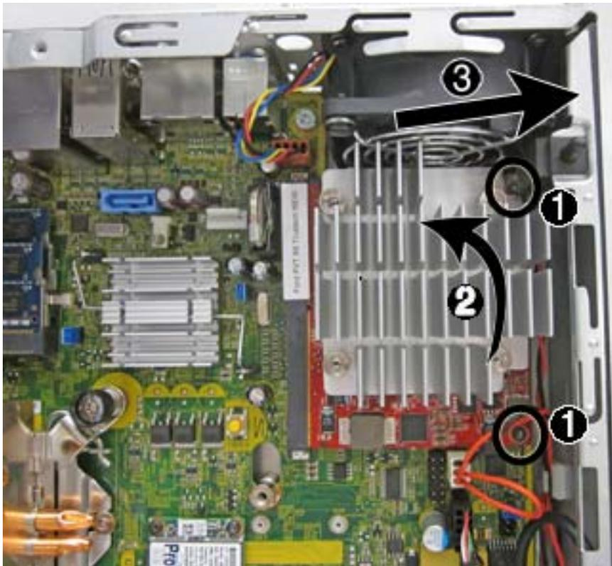
To install the graphics board, reverse the removal procedure.
