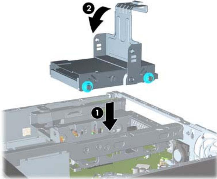
11. Replace the optical drive and reconnect the cable on the back of the optical drive.
