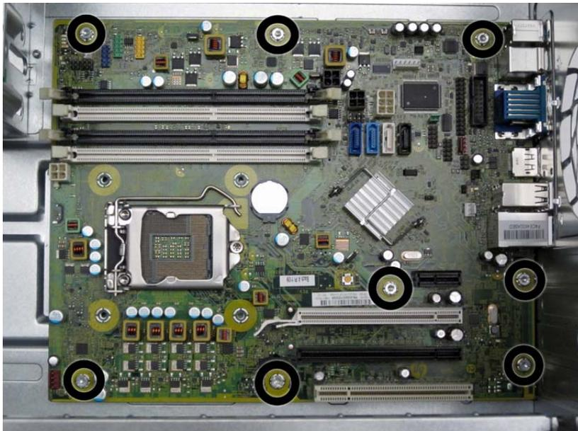
8. Slide the system board toward the front of the computer to disengage the I/O panel (1), lift the rear of the system board up at an angle (2), and then lift the system board out of the computer (3).
