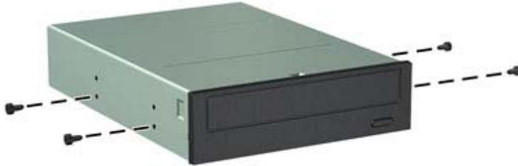
5. Position the guide screws on the drive into the J-slots in the drive bay. Then slide the drive toward the front of the computer until it locks into place.
