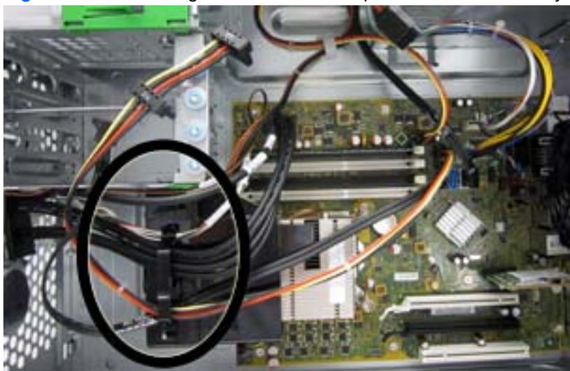
4. Unplug the fan cable from the system board connector labeled CHFAN.
