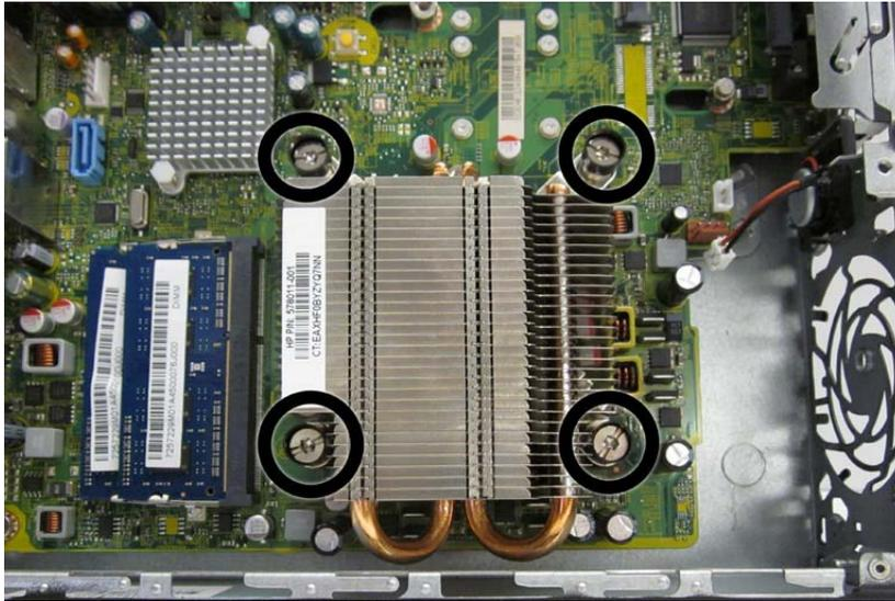
**⚠ CAUTION:** Heat sink retaining screws should be removed in diagonally opposite pairs (as in an X) to even the downward forces on the processor to avoid damage that could require replacing the system board.
