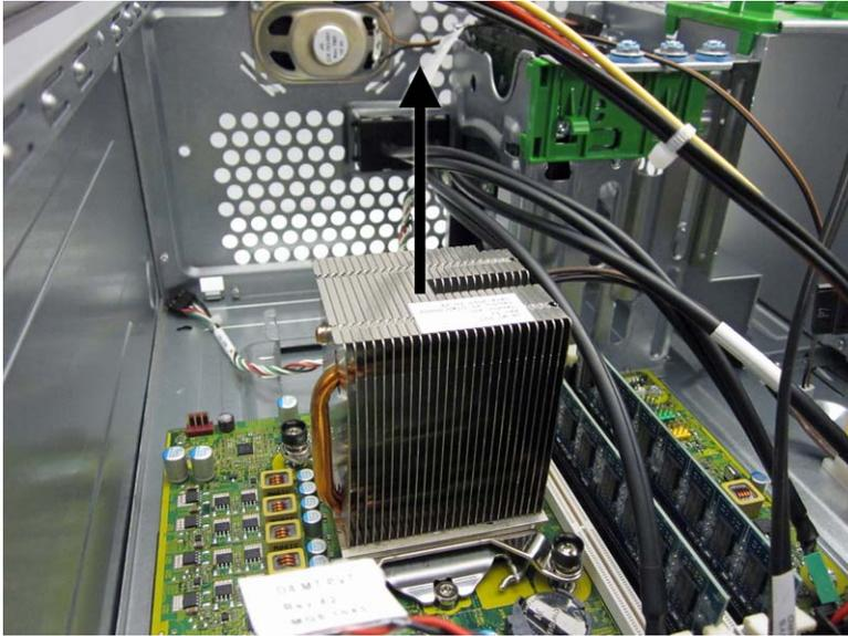
When reinstalling the heat sink, make sure that its bottom has been cleaned with an alcohol wipe and fresh thermal grease has been applied to the top of the processor.
