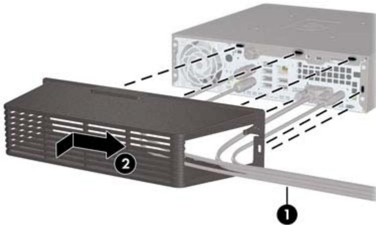
**NOTE:** For security purposes, you can install an optional cable lock to the chassis that locks the port cover and secures the computer.
