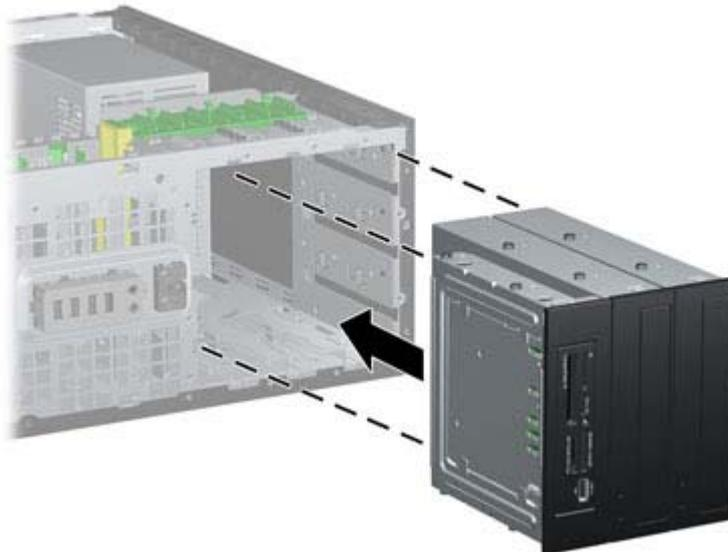
**CAUTION:** The bottom 5.25-inch drive bay has a shorter depth than the upper two bays. The bottom bay supports a half-height drive or other device that is no more than 14.5 cm (5.7 inches) in depth. Do not try to force a larger drive, such as an optical drive, into the bottom bay. This could cause damage to the drive and the system board. The use of unnecessary force when installing any drive into the drive bay may result in damage to the drive.
