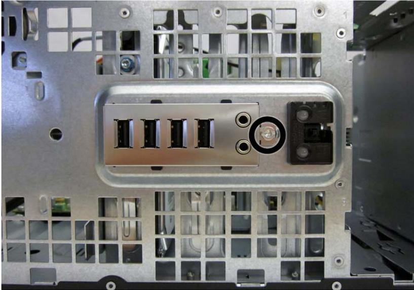
6. Rotate the right side of the assembly away from the chassis.
