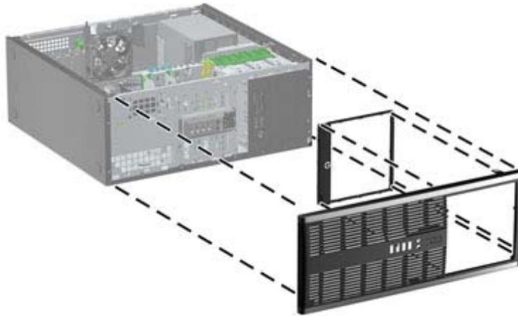
14. Replace the front bezel and computer access panel.
