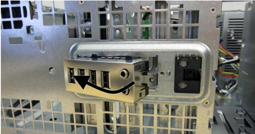
7. Pull the assembly toward the right and away from the chassis while threading the wires through the slot between the drive cage and chassis front and the hole in the front of the chassis.
