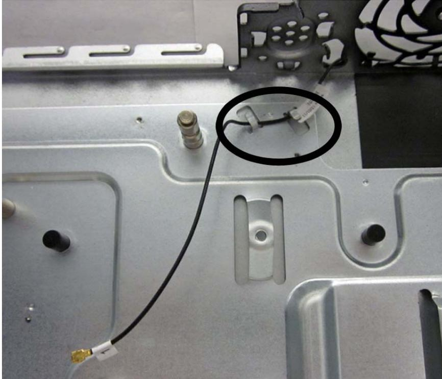
11. From the outside of the front of the chassis, remove the two Torx T8 screws (1) that secure the antenna to the chassis.
