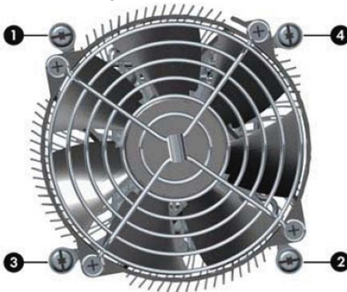
4. Disconnect the fan cable from the white system board connector labeled CPUFAN (1).
