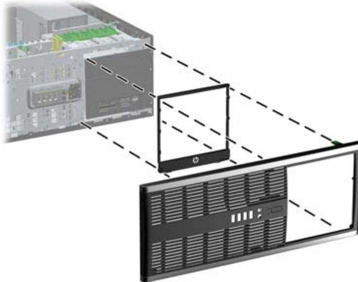
14. Replace the front bezel and computer access panel.
