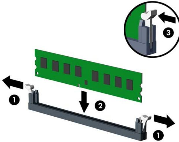
**NOTE:** A memory module can be installed in only one way. Match the notch on the module with the tab on the memory socket.
