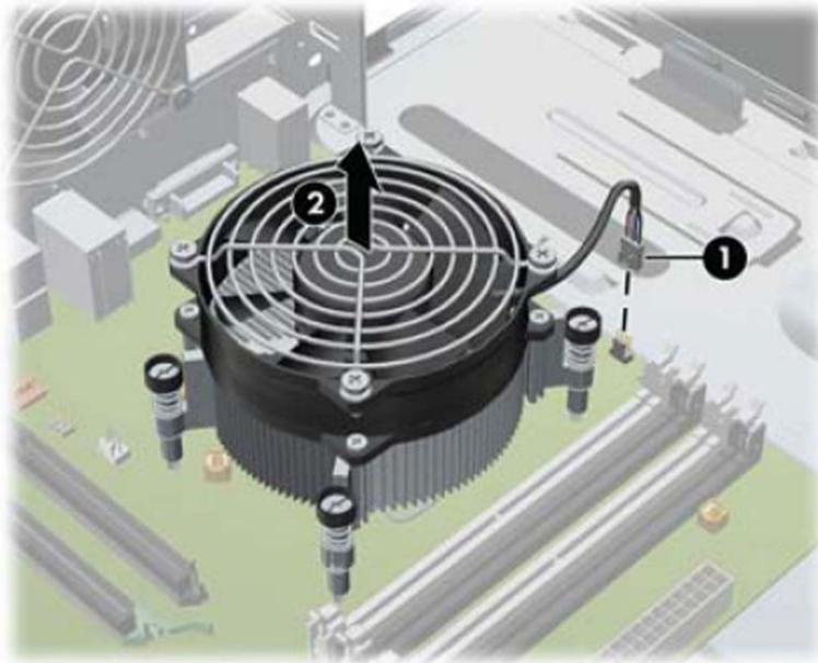
When reinstalling the fan sink, make sure that its bottom has been cleaned with an alcohol wipe and fresh thermal grease has been applied to the top of the processor.
