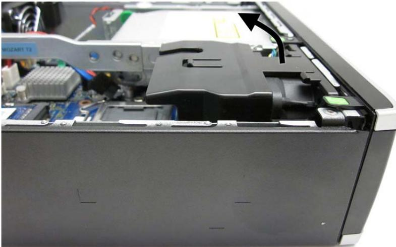
To install the front fan, reverse the removal procedure.
