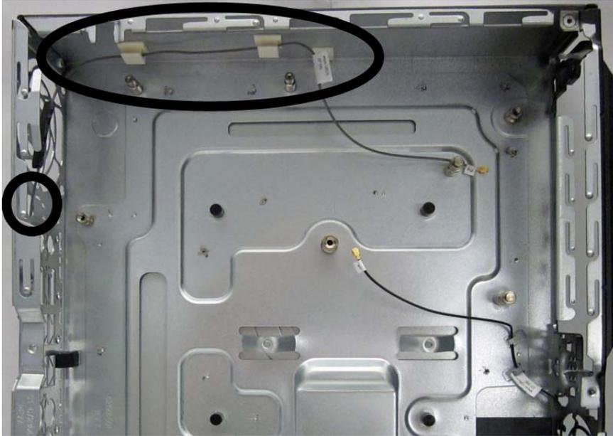
14. From the outside of the rear of the chassis, remove the two Torx T8 screws that secure the antenna to the chassis.
