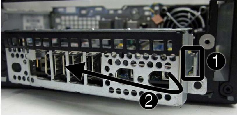
12. Remove the three remaining Torx T15 screws (1) that secure the system board to the chassis.
