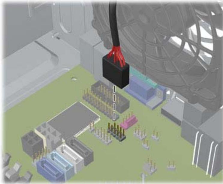
8. If installing a new drive, connect the opposite end of the data cable to the appropriate system board connector.
