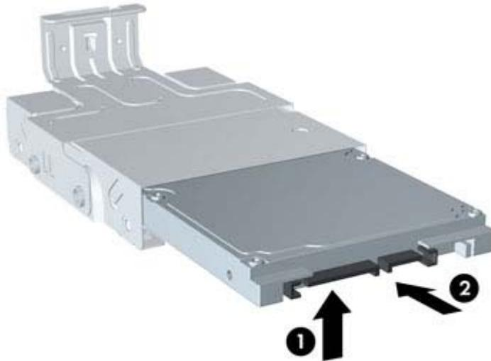
9. Set the hard drive down into the bottom of the carrier (1), then replace the four guide screws on the sides of the carrier to secure the drive in the carrier (2).
