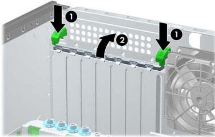
5. Before installing an expansion card, remove the expansion slot cover or the existing expansion card.
