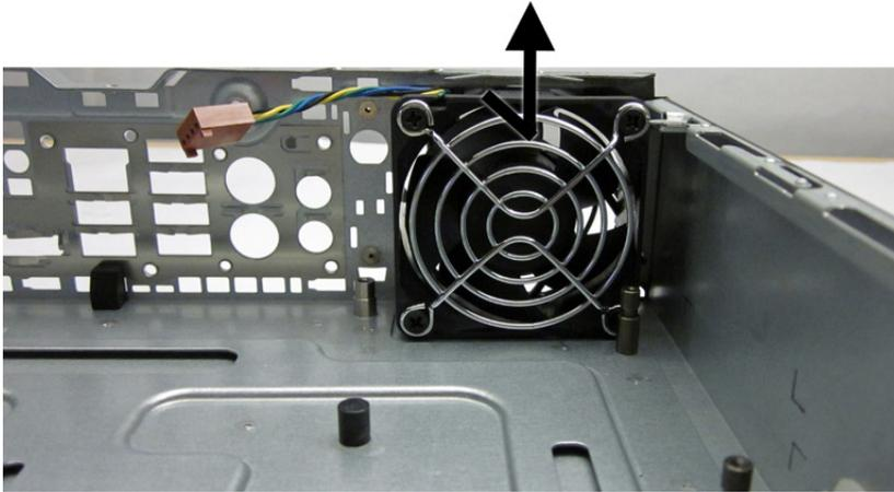
To install the rear fan, reverse the removal procedure.
