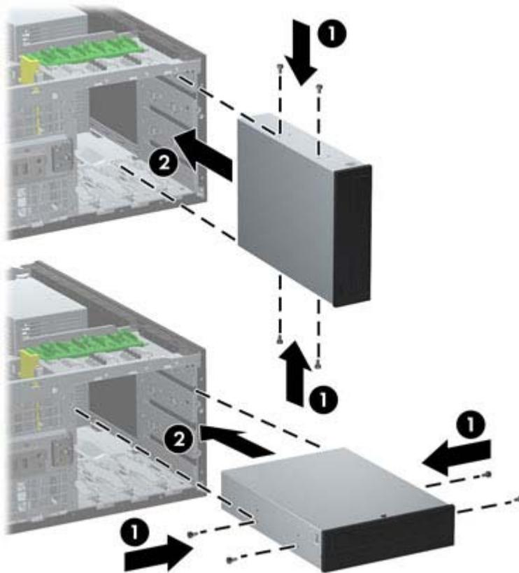
6. Install the drive in the desired drive bay by sliding it all the way into the front of the drive cage until it locks (2). The drivelock automatically secures the drive in the bay.
