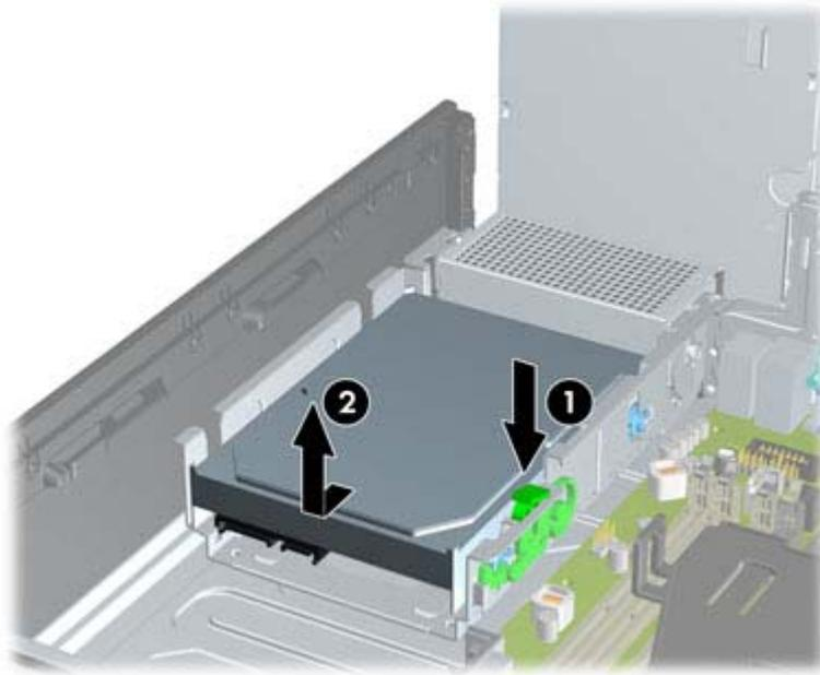
7. To install a hard drive, you must transfer the silver and blue isolation mounting guide screws from the old hard drive to the new hard drive.
