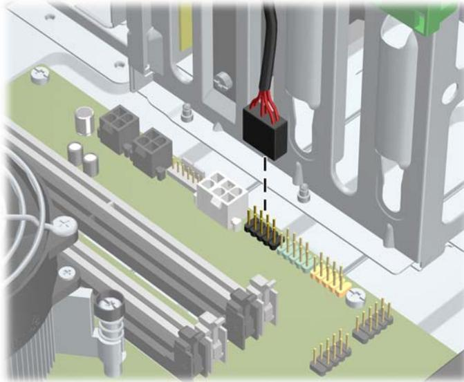
8. If you are installing a new drive, connect the opposite end of the data cable to the appropriate system board connector.
