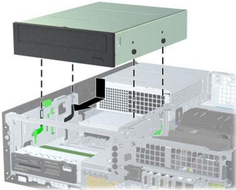
6. Rotate the drive cage to its upright position.
