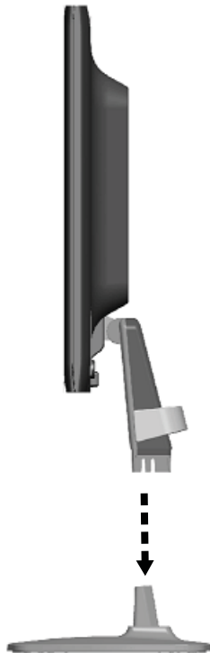
Figure 2-1 Assembling the ZR2040w pedestal
