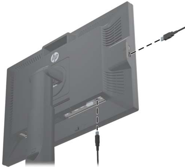
Figure 2-11 Connecting USB Cables
