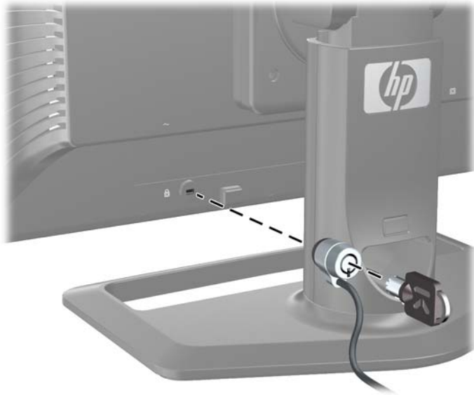
Figure 2-19 Installing a Cable Lock
