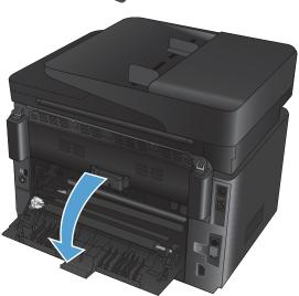
Remove any jammed paper. Use both hands to pull out the paper to avoid tearing.
