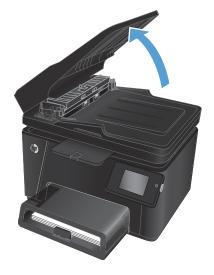
Use a moist, lint-free cloth to wipe both pickup rollers and the separation pad to remove dirt.
