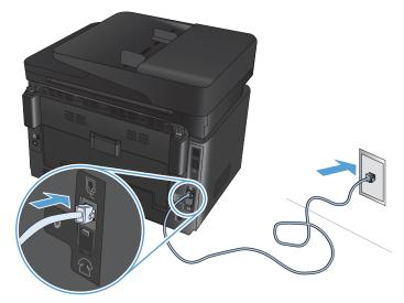
2. (Optional) To connect an answering machine or extension phone, pull down the rubber plug from the telephone port on the product. Connect another telephone cable to the telephone port on the product and to the "line in" port on the answering machine or extension phone.
