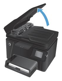
2. Use a moist, lint-free cloth to wipe both pickup rollers and the separation pad to remove dirt.
