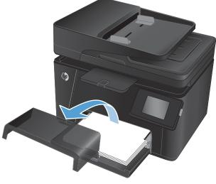
Remove the stack of paper from the input tray.
