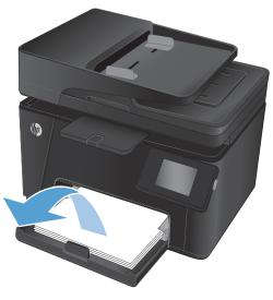
Remove any jammed paper visible in the input tray area. Use both hands to remove jammed paper to avoid tearing the paper.
