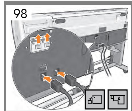
**EN** Plug the 2 power cables into the rear of the printer, and then plug the other ends of the 2 cables into the AC power outlet. Check the current circuit breakers are in the up position.
