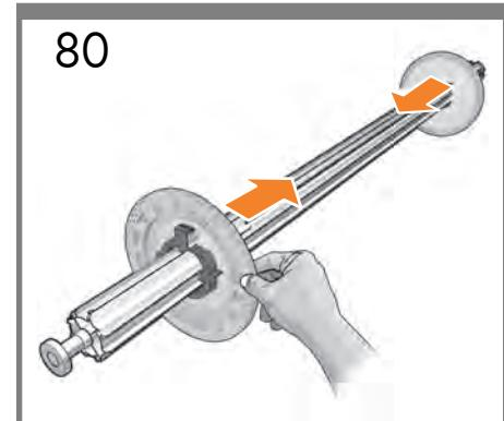
Slide the 2 hubs onto the spindle.
