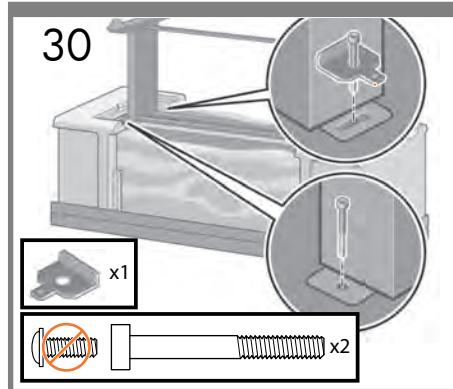
**EN** Use 2 screws to attach the left side of the stand to the printer. Attach the metallic plate as shown. Make sure that the screws are fully tightened.
