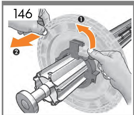
**EN** Unlock and remove the blue hub from the left end of the spindle. Keep the spindle horizontal.
