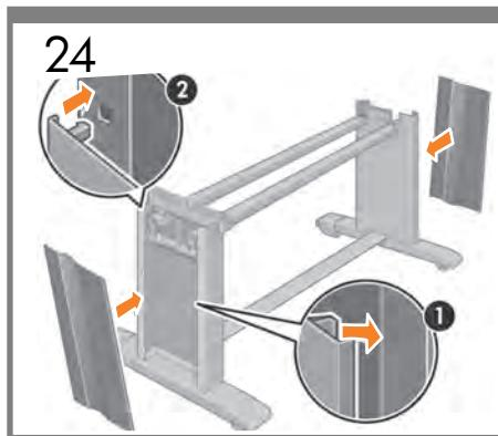
**EN** Position the left and right leg covers on the front of the legs (1), and then clip the rear edge (2) into place. Note: both covers are the same.
