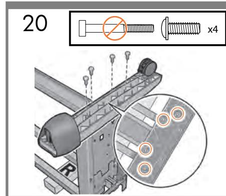
Use 4 screws to attach the foot to the right leg. Tighten each screw around five times, and then gradually tighten each screw completely.
