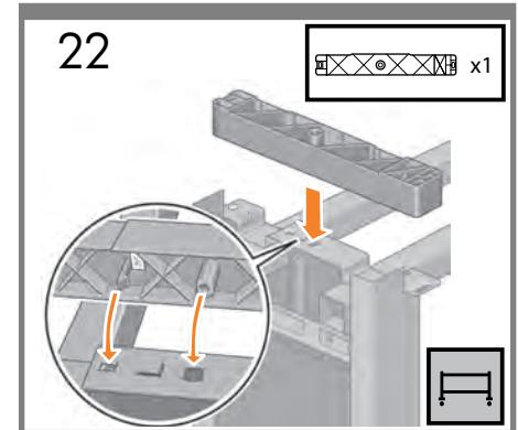
Attach the left stand spacer to the top of the left leg. It will "click" into place.
