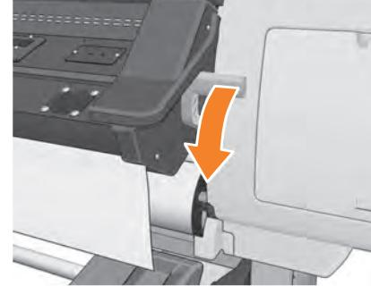
**EN** Lower the substrate-adjustment lever.
