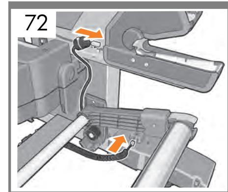
**EN** Connect the sensor cable to the rear of the take-up reel module. Connect the sensor cable to the sensor unit located on the right foot. Note: This is connected at the back of the printer.
