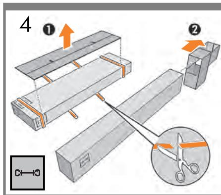
**EN** Cut the straps, and separate the boxes shown.
