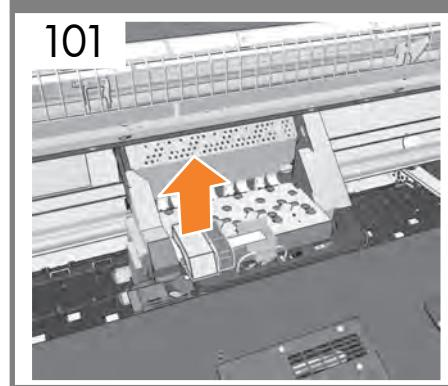
Open the window. Remove the packing foam from the top of the printhead carriage. Close the window.
