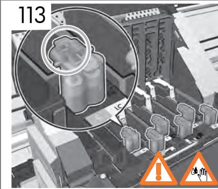
Do not remove the setup printheads yet. Look at each printhead and verify that each printhead contains ink.
