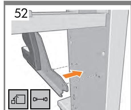
**FR** Locate the 2 pins on the take-up reel left hand module into the holes on the left leg.
