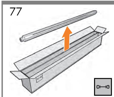
**EN** Carefully lift the take-up reel assembly. The central core tube contains the take-up reel spindle.
