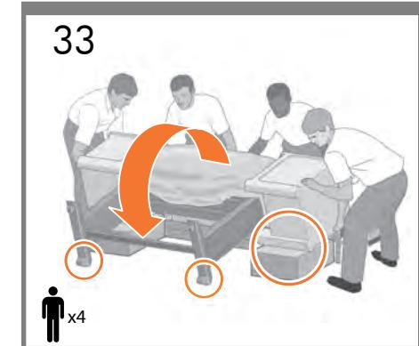
**EN** Rotate the printer until the back of the printer rests on the spare box and the supplies box.
