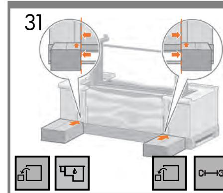
**EN** Place the take-up reel box and the supplies box against the rear of the printer box. The arrows on the boxes must point towards the printer box. Make sure that the anti-slip material is attached to the 2 rear wheels.
