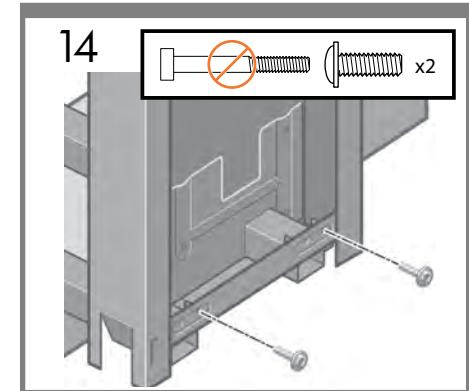
**EN** Use 2 screws on the outside of the right leg to attach the left leg to the cross-brace.
