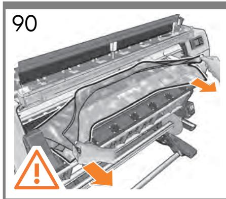
**Pull the plastic sheet out carefully. Note: If by accident any particles fall on the printzone or carriage rod proceed to clean and lubricate the rod.**
