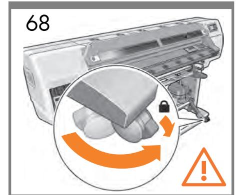
**EN** Move the front right wheel so that it faces forward, and then lock it into place.
