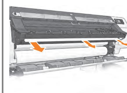
**EN** Wait until the substrate emerges from the printer as shown.
