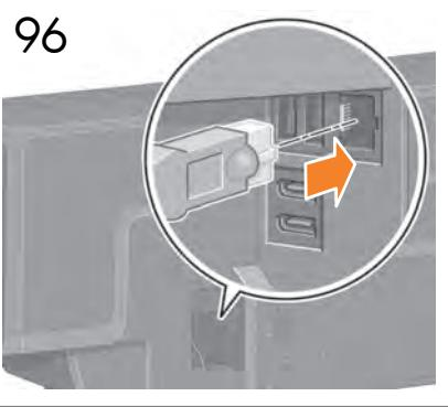
**EN** From the rear of the printer; plug the Gigabit Ethernet cable into the Gigabit Ethernet connection.
