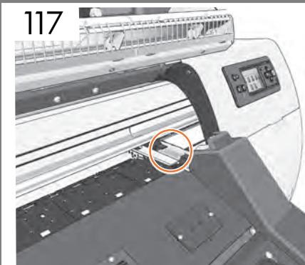
Wait until the front panel indicates to, then open the window and locate the ink funnel entrance.
