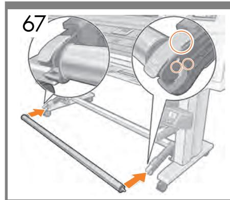
**EN** Slot the loop shaper bar into place.
