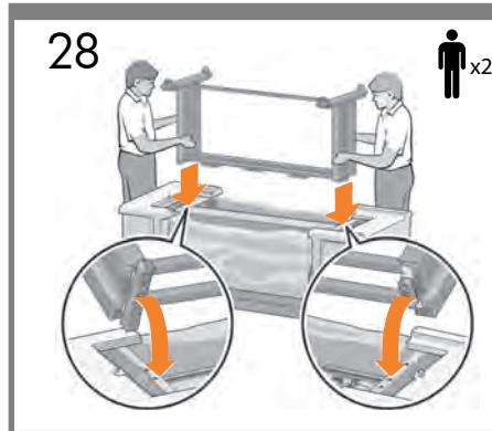
Lift the stand assembly onto the printer engine. The anti-slip material should face the rear of the printer (the rear is the black flat side with a yellow sticker). Check that the tube from container does not interfere with the stand and printer.
