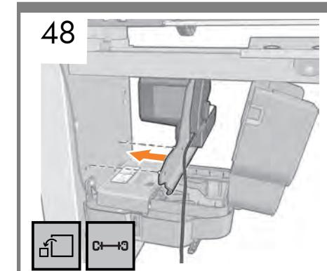
**Carefully locate the take-up reel module into place by inserting the 2 pins. Note: if required, open the waste management unit lid in order to access the screw holes. Take care not to let the module fall onto the waste management unit below.**
