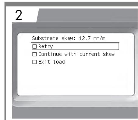
If the substrate is loaded with a skew, select Retry to reload the substrate and eliminate the skew.
