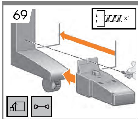
**EN** Slide the sensor unit onto the right foot, and then use the screw shown to attach the unit.
