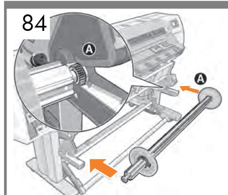
**EN** Load the take-up reel spindle into the printer by pushing firmly on each end of the spindle. Note: the part marked A should go to the right hand side.
