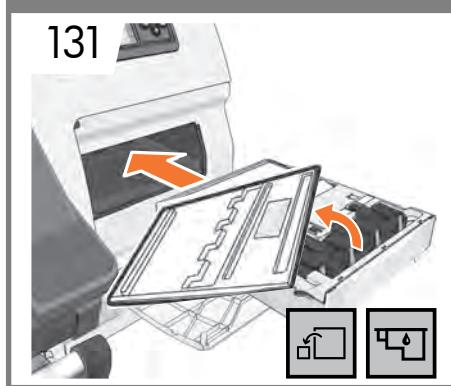
**EN** Remove the transparent shipping tray. Insert the maintenance cartridge, pushing it in and down until it clicks into place, and then close the maintenance cartridge door and press OK in the front panel.
