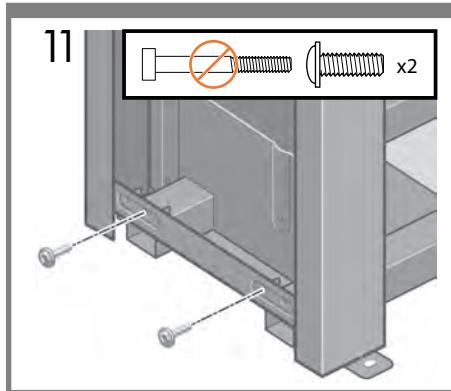
**EN** Use 2 screws on the outside of the left leg to attach the left leg to the cross-brace.
