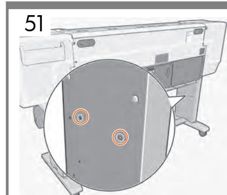
**FR** Identify the 2 holes on the inside of the left leg. The holes are used to attach the left side of the take-up reel assembly.
