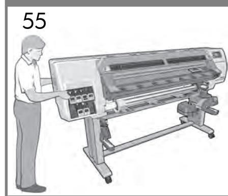
**IMPORTANT:** Move the printer to its final location. Once the take-up reel sensor is installed, the wheel is locked.
