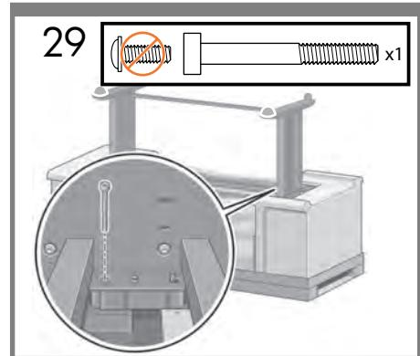
Use 1 screw to attach the right side (if in doubt, this is the only side that has a hole) of the stand to the printer engine. Make sure that the screw is fully tightened.
