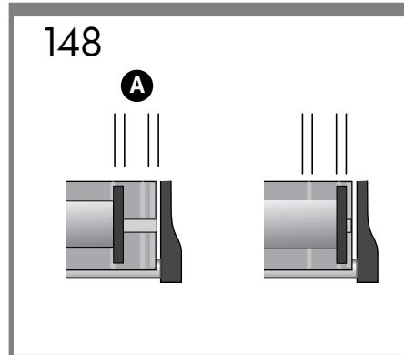
**EN** The right hub of the spindle has 2 positions: 1 for rolls of the printer's maximum width, and another for narrower rolls. Note: in order to move the hub, squeeze the 2 blue pieces. A = preferred position when possible.
