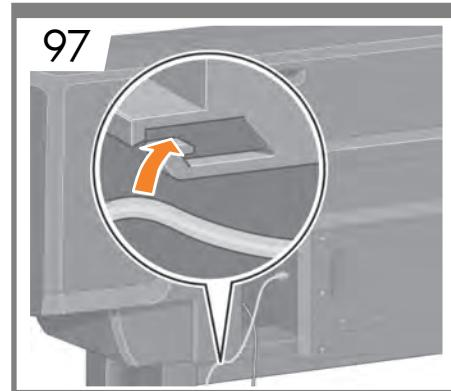
**EN** Pass the Gigabit Ethernet cable through the hook at the rear of the printer.
