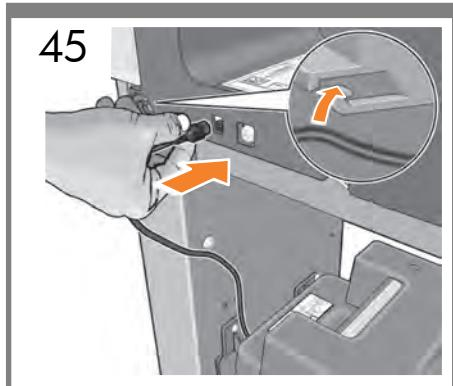
**EN** Plug the cable into the rear. Pass the cable through the hook at the rear of the printer.
