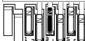
**EN** If a "Reinsert" message appears on the front panel, then firmly reseat the printheads. If the problem persists, refer to the Maintenance and troubleshooting guide.
