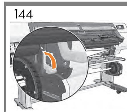
Remove the adhesive tape, and lift the spindle lock lever to disengage the spindle.
