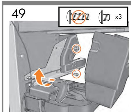
**EN** Attach the take-up reel module to the stand with 3 screws.
