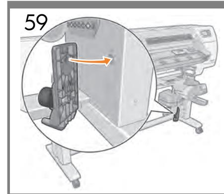
**Locate a pivot block onto the right hand leg.**
