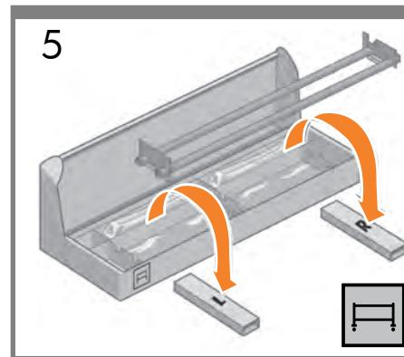
**EN** Open the box that contains the stand. Remove the 2 boxes marked L and R. Place them on the floor as shown.
