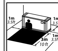
**EN** The space required for assembly is 3m (10 feet) in front and 1m (3.5 feet) at the sides and rear.
