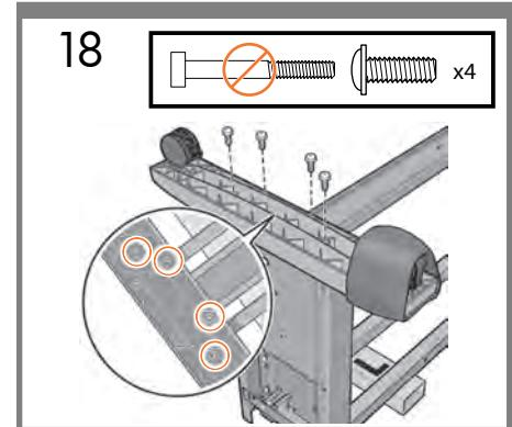
Use 4 screws to attach the foot to the left leg. Tighten each screw half-way, and then gradually tighten each screw completely.
