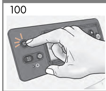
If the power light on the front panel remains off, press the Power button to switch on the printer.
