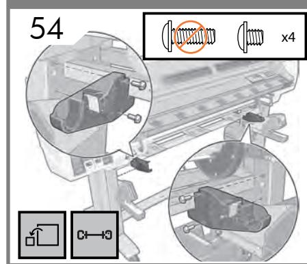
**EN** Use 4 screws to attach the loading table supports.
