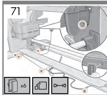
**EN** Insert the 6 clips provided into the positions shown.
