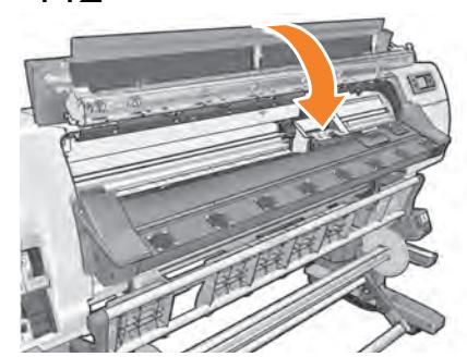
Close the printer window and secure the latches.
