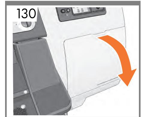
**EN** Pull open the printhead cleaning cartridge door, which is located on the right side of the printer.
