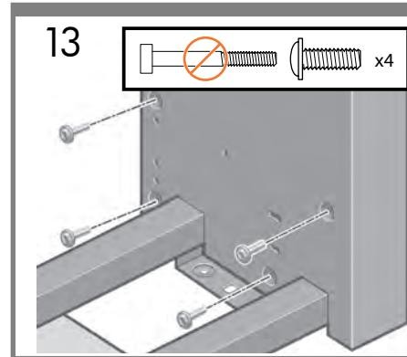
**EN** Use 4 screws on the inside of the right leg to attach the right leg to the cross-brace.
