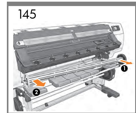
Remove the spindle from the printer.
