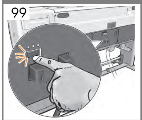
**EN** Turn the power switch to the On position at the rear of the printer.
