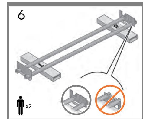
**EN** Lower the left side of the cross-brace onto the box marked L and the right side of the cross-brace onto the box marked R.
