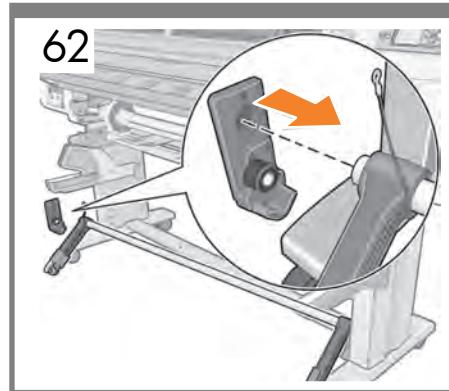
**EN** Locate a pivot block onto the left hand side of the loop shaper.
