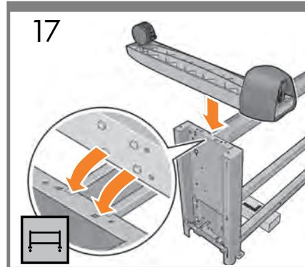
Place a foot on the left leg. There are pins to help you correctly position the foot. Do not remove the anti-slip material from the wheel.
