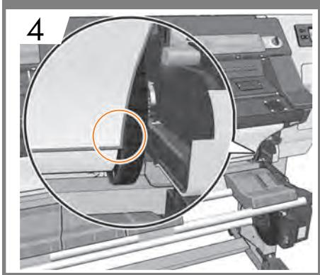
**EN** Align the substrate with the edge of the roll.
