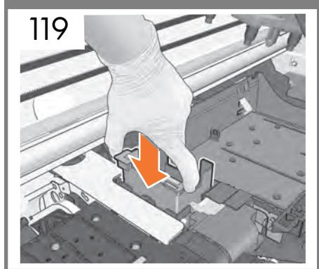
**EN** Feed the assembly tube all the way in, and then slot the piece at the end into the hole as shown.
