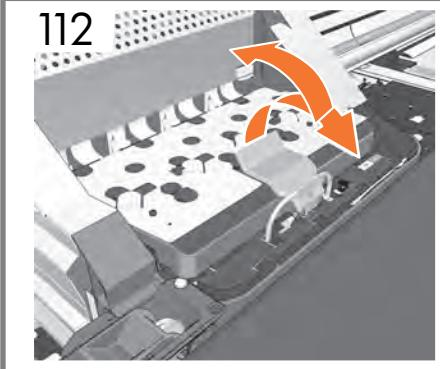
Pull up and release the blue latch on top of the carriage assembly. Lift the blue latch to open the printhead cover.
