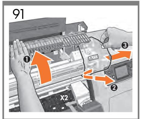
**Lift up the isolator grill (1), remove the tapes (2), and pull the plastic bags out (3). Ensure that both plastic bags are removed. Note: If by accident any particles fall on the printzone or carriage rod proceed to clean and lubricate the rod.**
