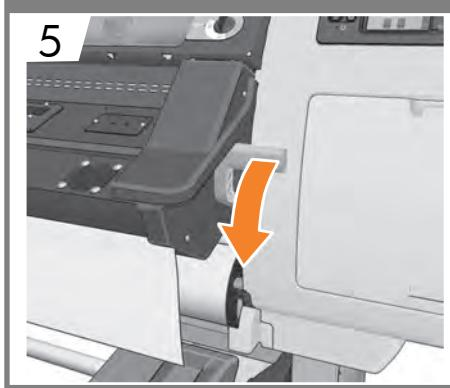
**EN** Lower the substrate-adjustment lever.
