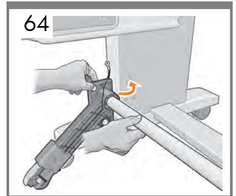
**EN** Slide the pivot block into the 3 holes.
