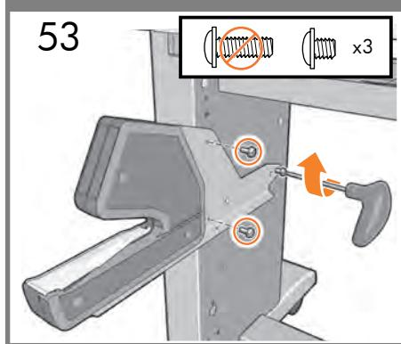
**EN** Attach the left side take-up reel module with 3 screws.
