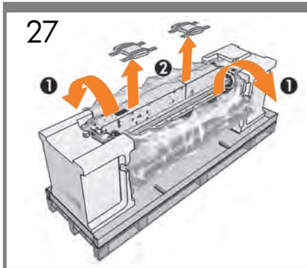
Pull open the protective plastic from the base of the printer (1), and then remove the 2 desiccant bags (2).
