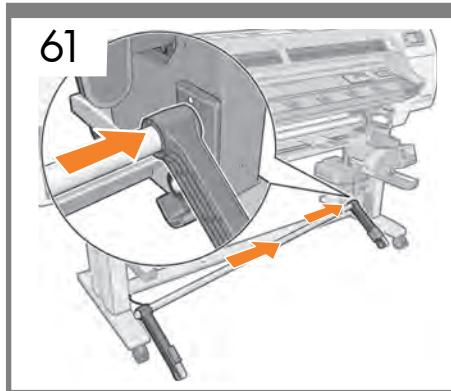
**EN** Insert the loop shaper into the right hand side pivot block.
