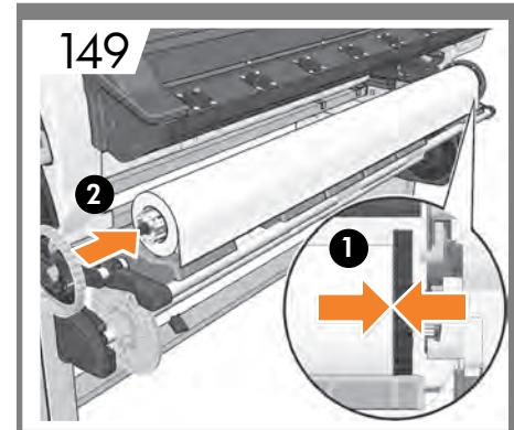
**EN** Fully insert the spindle into the substrate roll (No gap should exist between the spindle hub and the roll).
