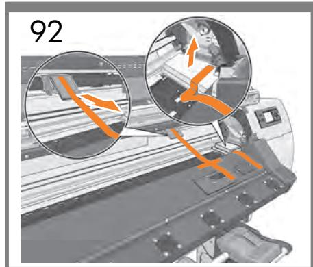
**EN** Remove the protective packaging from inside the printer; cut the tape if needed.
