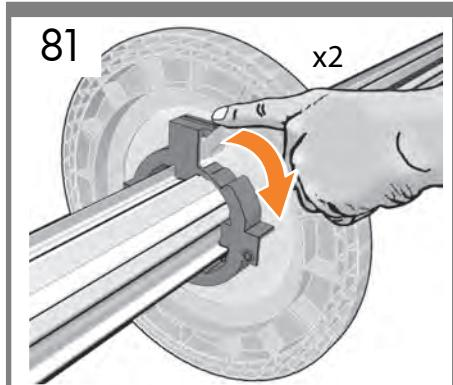
**EN** Lock the hubs. Note: you can adjust the hub when loading media.
