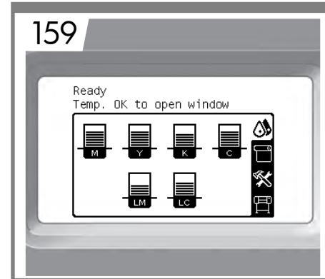
**EN** The printer automatically performs substrate advance calibration and printhead alignment. Please do not stop those processes to ensure successful PH alignment.
