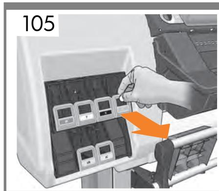
To release the ink cartridge drawer, gently pull down on the blue handle, and then slide out the ink cartridge drawer.
