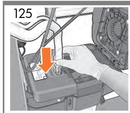
**DE** Insert the tube end into the slot. Note: it may be difficult to insert the tube correctly, you may have to turn the tube so that it enters.
