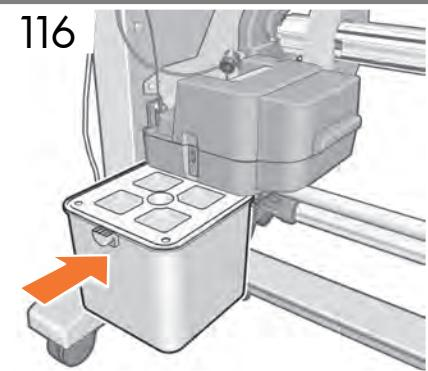
Slide the printhead cleaning container onto the guides, and push it all the way in.
