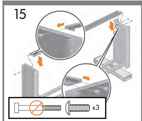
**EN** Use 3 screws to attach the cross-bar to the legs. Note: the bar can only fit one way; at one end there is 1 hole, at the other 2.
