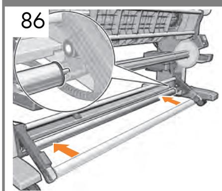
Note: If you are not using the loop shaper, you can either store its parts in a safe place, or in the park position shown.
