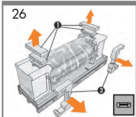
**EN** Remove the 4 packing pieces from the top and 2 pieces from the side as shown.
