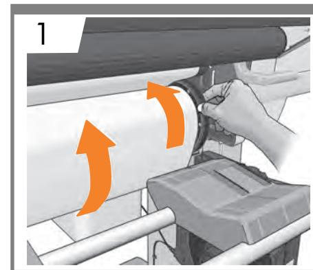
**EN** Use the hubs to wind the excess substrate onto the spindle if the front panel requests you to do so.
