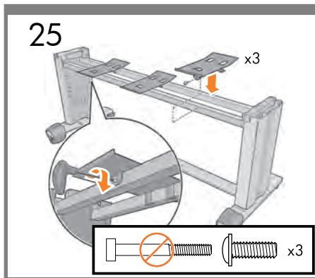
**EN** Attach the 3 deflectors to the top of the stand using 1 screw for each.
