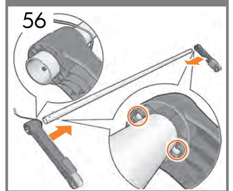
**Locate the 2 loop shaper arms onto the shaft, slotting them onto the pins. Make sure that both blue locks face the same direction: up or down.**
