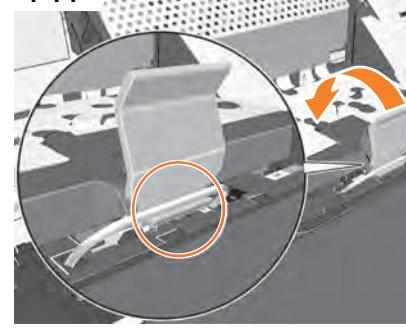
Lower and lock the blue latch. Make sure that the blue latch is correctly engaged, and then lower the latch.
