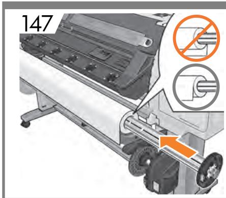
**EN** Rest the roll of substrate that you want to load on the loading table. Note: make sure that the roll is placed correctly as shown above.
