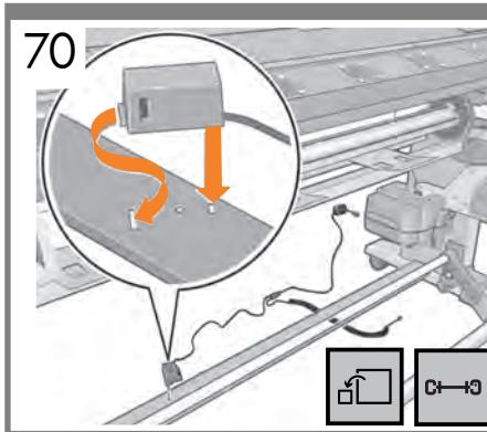
**EN** Attach the sensor unit onto the left side of the lower cross-brace.
