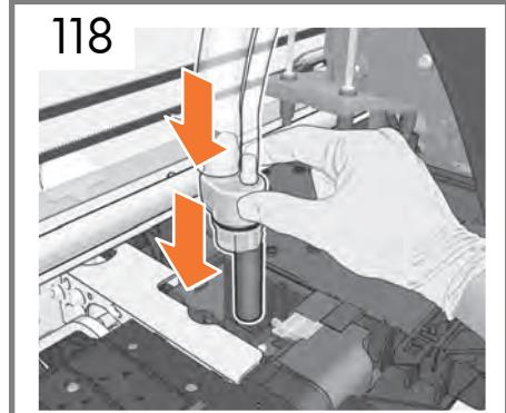
Insert the tube assembly, orientated as above, into the Drop Detector.
