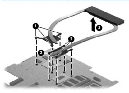
b. Thoroughly clean the thermal connections (1) and (3) on the system board and the heat sink (2) and (4) before replacing a heat sink onto a system board. Continue to step 3.
