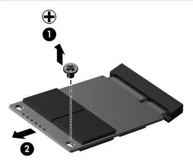
Reverse this procedure to install the mSATA drive onto a replacement system board.
