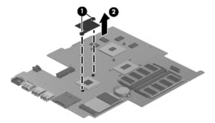
Reverse this procedure to install the PCH heat sink onto a replacement system board.
