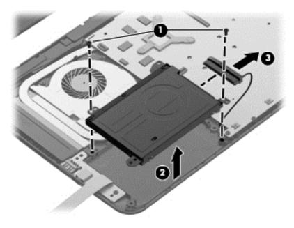
3. Remove the four Phillips screws (1), and then remove the bracket (2) from the hard drive.
