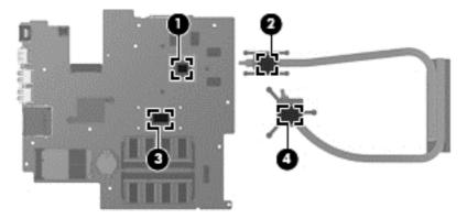
Loosen the captive screws (1) and lift the UMA graphics heat sink (2) from the system board.
