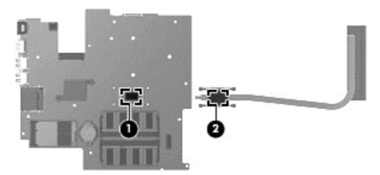
Reverse this procedure to replace the heat sink. Replace the thermal material that ships with the replacement heat sink.
