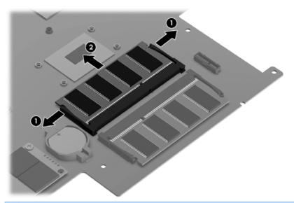
CAUTION: To protect a memory module after removal, place it in an electrostatic-safe container.
