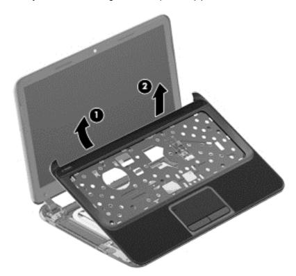
When replacing the top cover, be sure that the power button board and cable (see <u>Power button</u> <u>board on page 53</u>) are removed from the defective top cover and installed on the replacement top cover.
