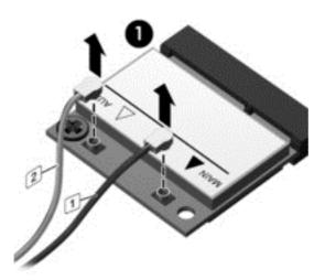
Remove the Phillips screw (2) that secures the WLAN module to the system board. (The WLAN module tilts up.)
