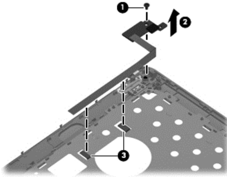
Reverse this procedure to install the power button board.
