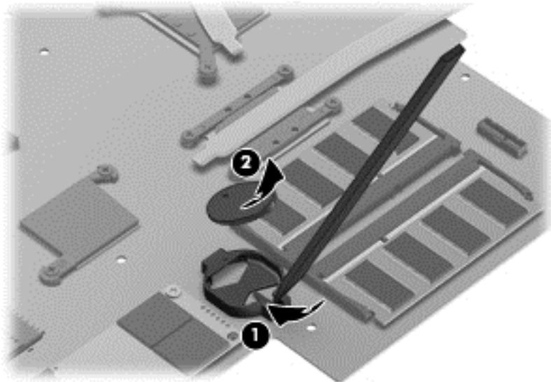
Reverse this procedure to install the RTC battery.
