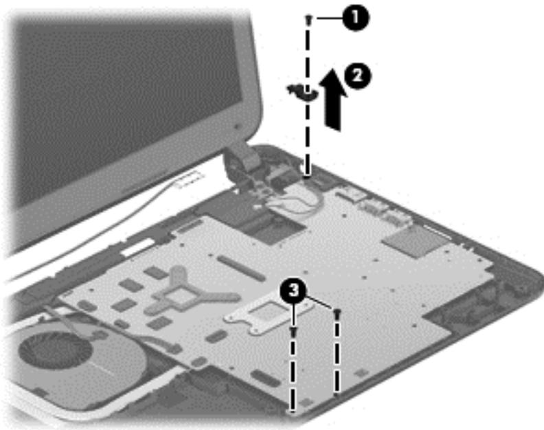
4. Lift the left side of the system board (1) until it rests at an angle.
