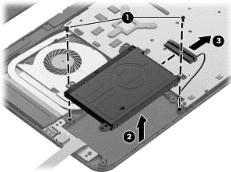
3. Remove the four Phillips screws (1), and then remove the bracket (2) from the hard drive.
