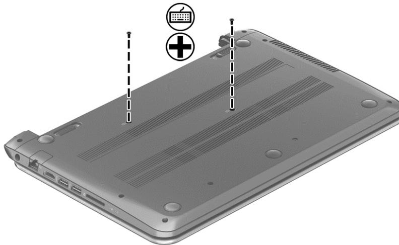
2. Turn the computer right-side up with the front toward you. Open the display and stand the computer on its right side. Insert a thin tool through the keyboard access hole. (The keyboard icon indicates the keyboard access hole.) Push firmly on the bottom of the keyboard until it disengages from the computer.
