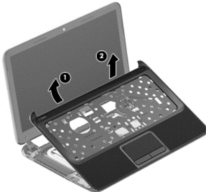
When replacing the top cover, be sure that the power button board and cable (see [Power button board on page 53](#)) are removed from the defective top cover and installed on the replacement top cover.
