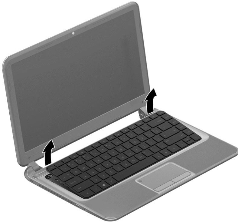
5. Tilt the keyboard forward (1) onto the palm rest. Release the zero insertion force (ZIF) connector (2) to which the keyboard cable is attached, and then disconnect the keyboard cable (3) from the system board.
