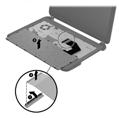
Reverse this procedure to install the keyboard.
