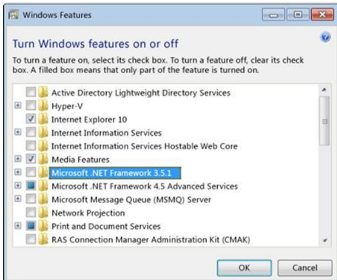
Figure F-2. Message box that allows you to turn on .NET Framework 3.5.1
