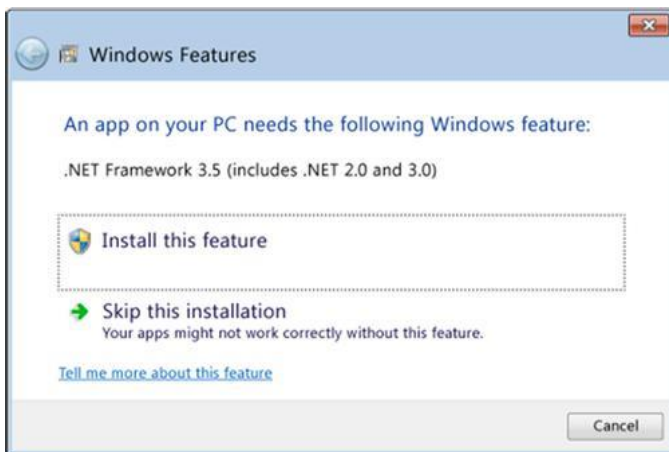
Figure F-1. Message box that allows you to install .NET Framework 3.5 on demand
