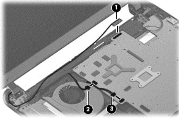
2. Remove the power connector bracket Phillips screw **(1)** and remove the power connector bracket **(2)**.
