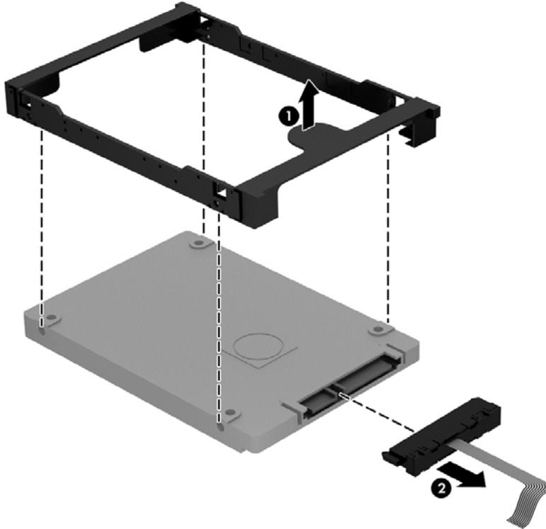
To install a hard drive, reverse this procedure.
