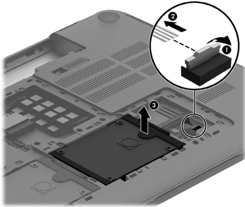
3. Lift the hard drive (3), and then slide it out of the hard drive bay.
