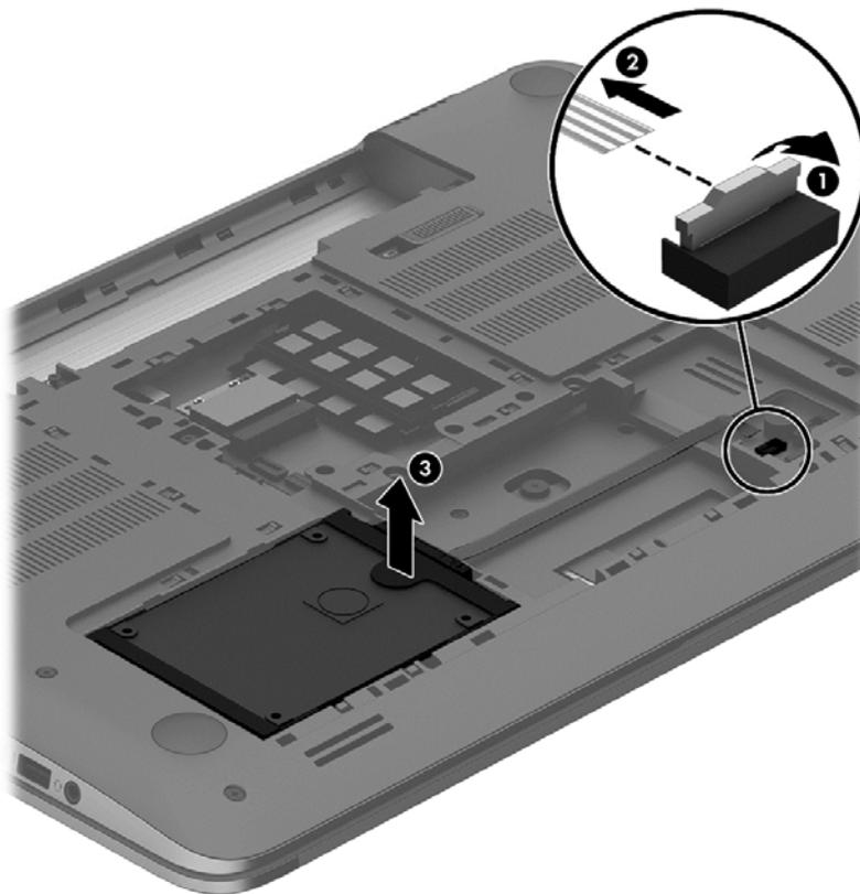
3. Lift the hard drive (3), and then slide it out of the hard drive bay.
