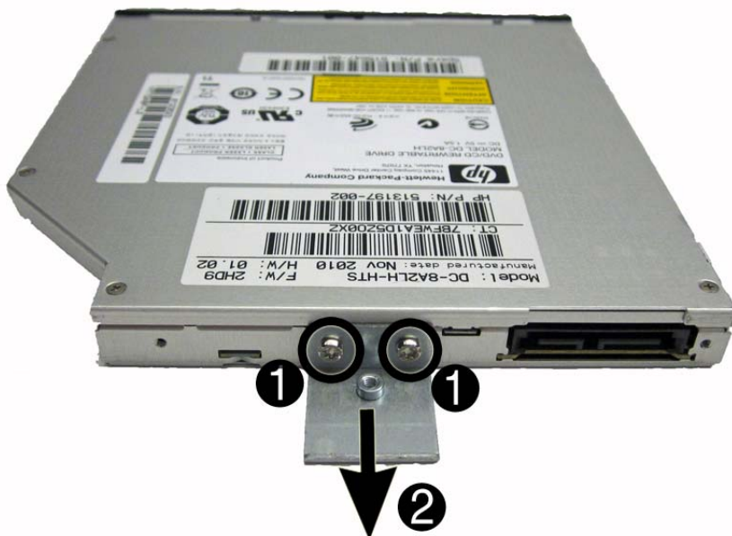
Figure 6-12 Removing the optical drive bracket
