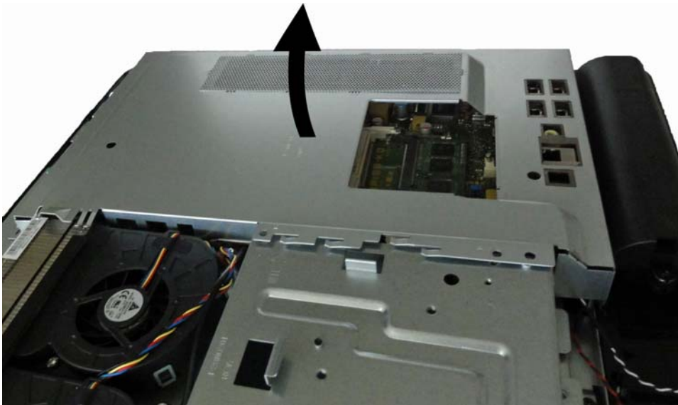
Figure 6-29 Removing the system board cover
