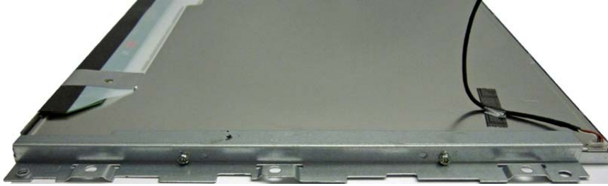
Figure 6-62 Samsung backlight cable and right panel bracket
