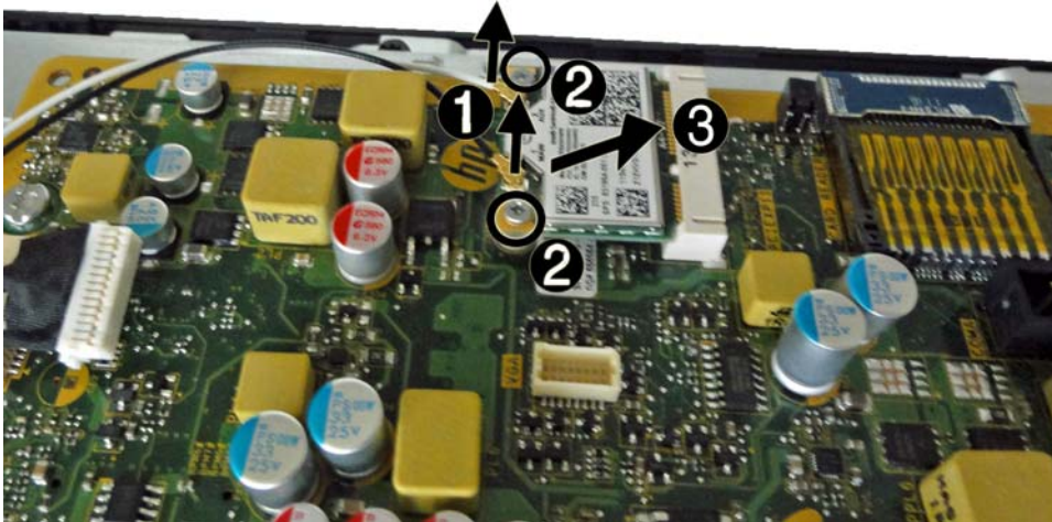
Figure 6-40 Removing the WLAN module
