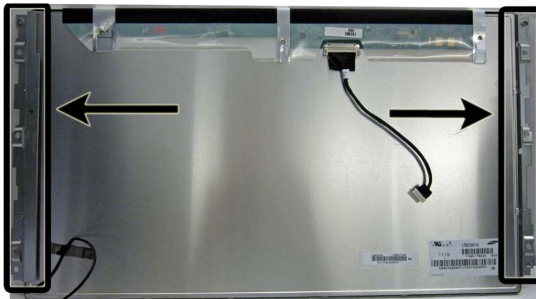
Figure 6-61 Samsung display cable and left panel bracket
