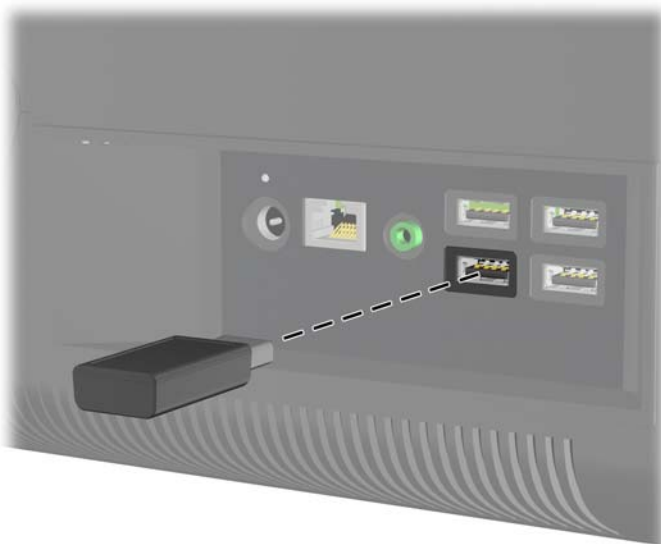
Figure 6-1 Installing the wireless receiver
