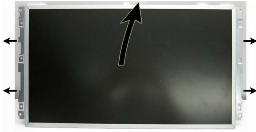
Figure 6-59 Removing the display panel – Samsung panel
