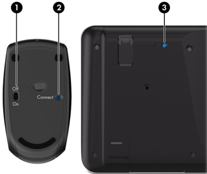
Figure 6-2 Synchronizing the wireless keyboard and mouse
