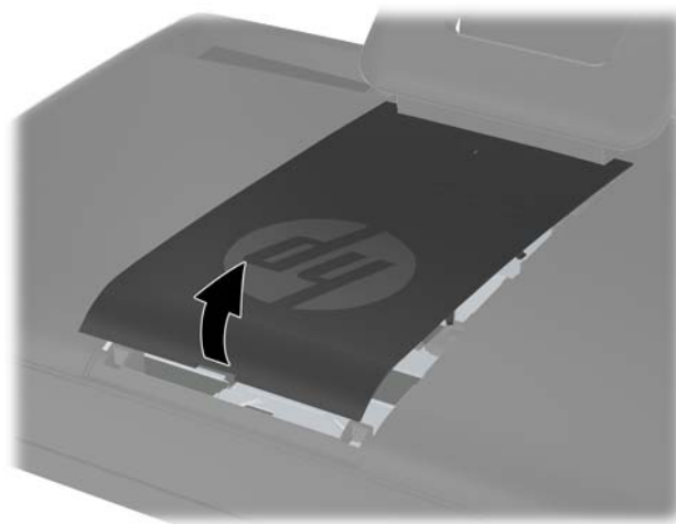
Figure 6-4 Removing the center access panel
